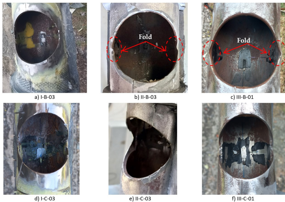
Figure 16: Localized buckling for samples of tubes from classes B and C.
