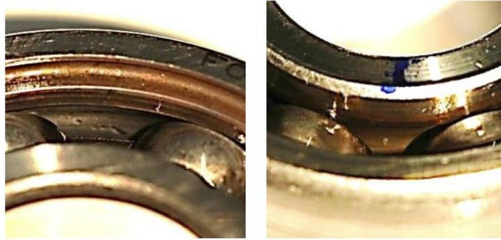
Figure 5. Faults of bearing running on fatigue accelerated life testing machine.
