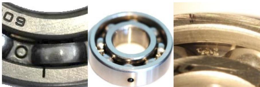
Figure 4. Artificially damaged bearings.
