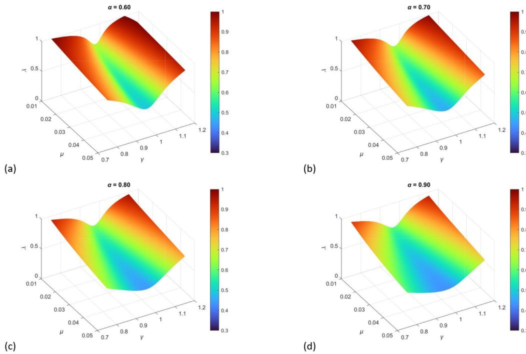
**Figure 12** Surfaces relating the structure displacement response ratio ( $\lambda$ ) for the El Centro earthquake to the parameters of mass ratio ( $\mu$ ) and tuning ratio ( $\gamma$ ), considering different values of aspect ratio ( $\alpha$ ): (a)  $\alpha = 0.60$  (b)  $\alpha = 0.70$  (c)  $\alpha = 0.80$  e (d)  $\alpha = 0.90$ .
