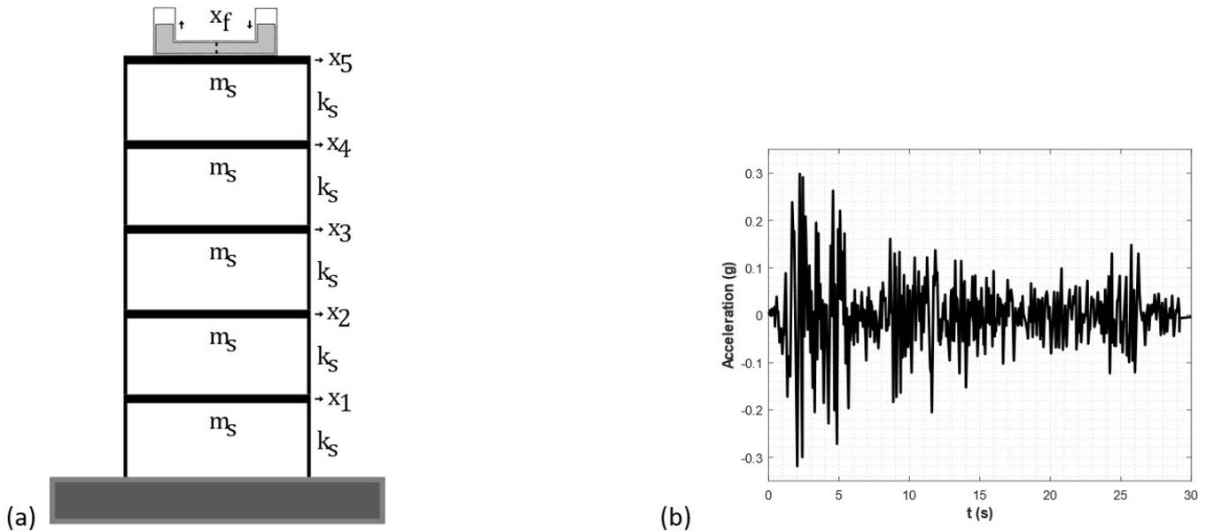
**Figure 11** (a) Five-story shear building with TLCD attached to the fifth story and (b) time history of ground acceleration for the El Centro earthquake
