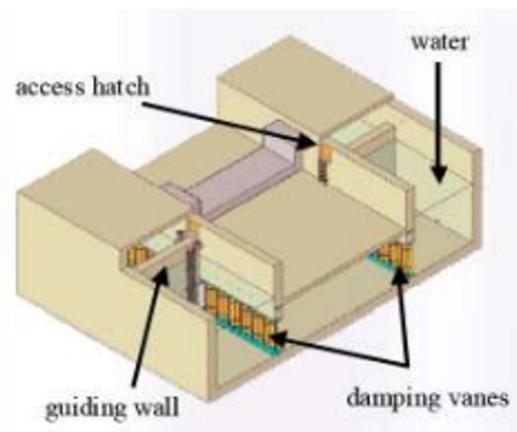
**Figure 1:** Application of a tuned liquid column damper (TLCD) in Comcast Center, Philadelphia, US (<https://www.dhuy.com/comcast-center-tuned-liquid-column-damper>). D'Huy Engineering, Inc. "Comcast Center - Tuned Liquid Column Damper". <https://www.dhuy.com/>. Accessed December 28<sup>th</sup>, 2022. <https://www.dhuy.com/comcast-center-tuned-liquid-column-damper>.
