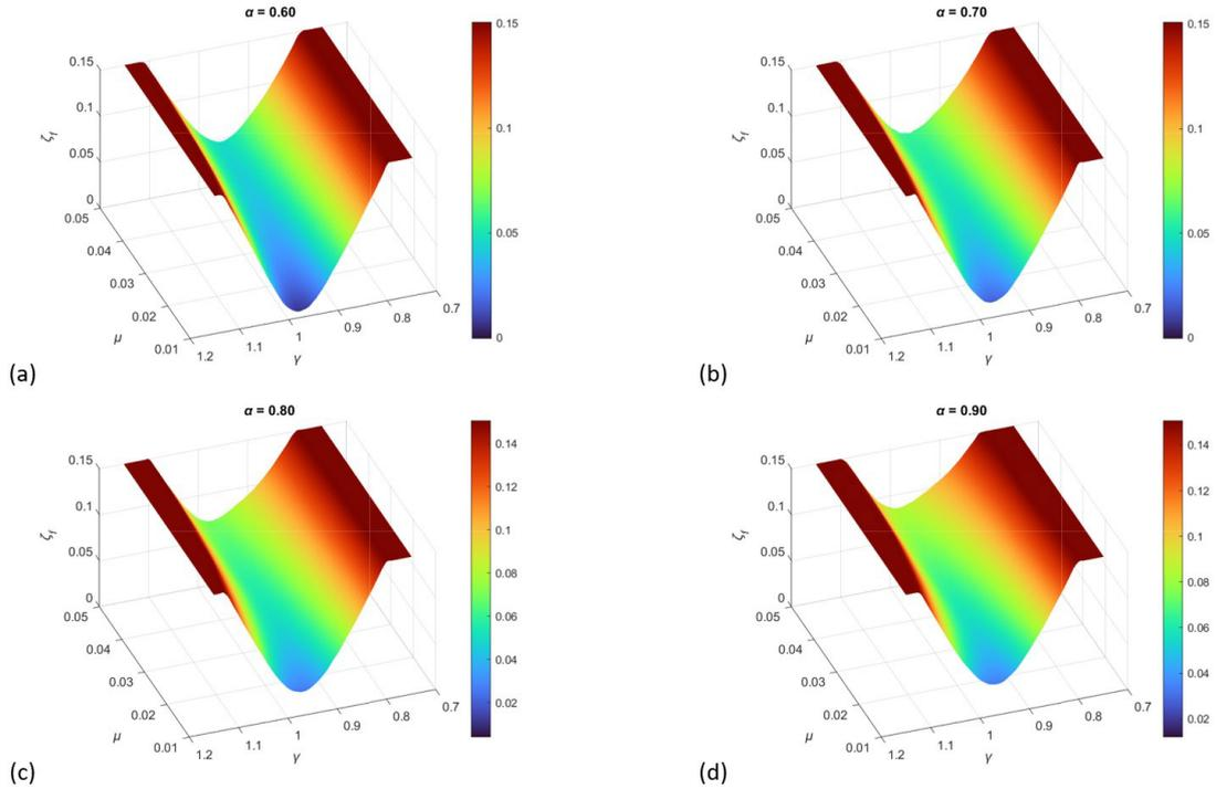
**Figure 14** Surfaces relating the TLCD damping ratio ( $\zeta_f$ ) to the mass ratio ( $\mu$ ) and tuning ratio ( $\gamma$ ) parameters, considering different values of aspect ratio ( $\alpha$ ): (a)  $\alpha = 0.60$  (b)  $\alpha = 0.70$  (c)  $\alpha = 0.80$  e (d)  $\alpha = 0.90$ .
