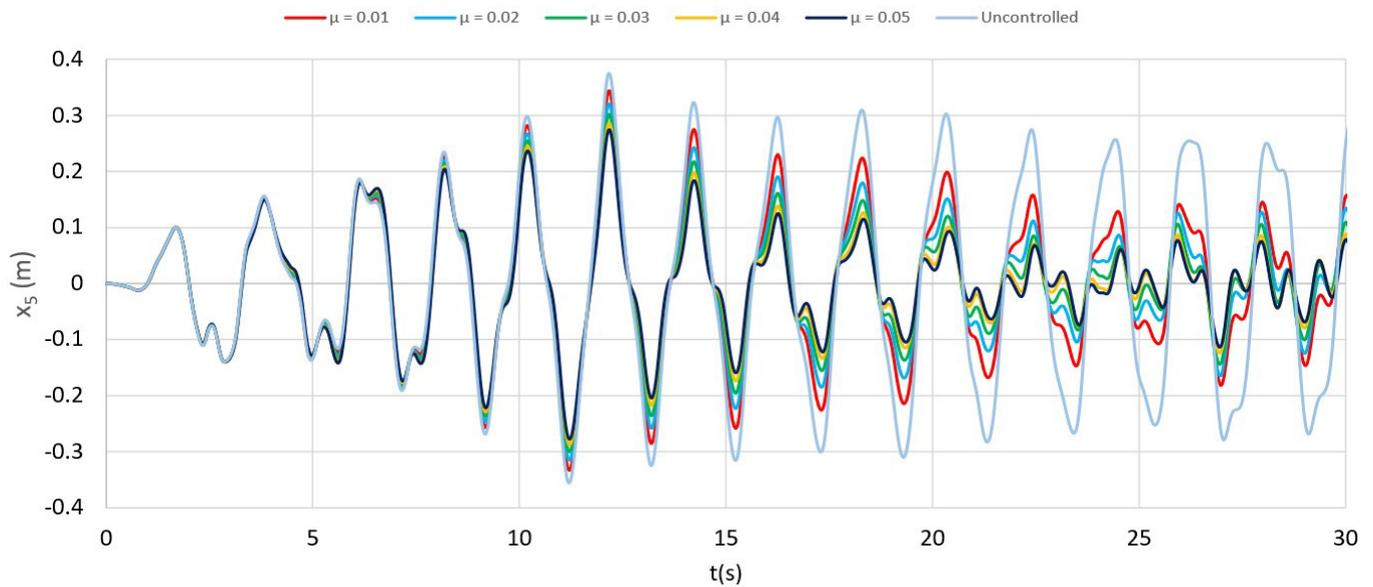
**Figure 16** Time response of the top of the structure ( $x_5$ ) with the mass ratio variation of the ideal TLCD designed from the response map.
