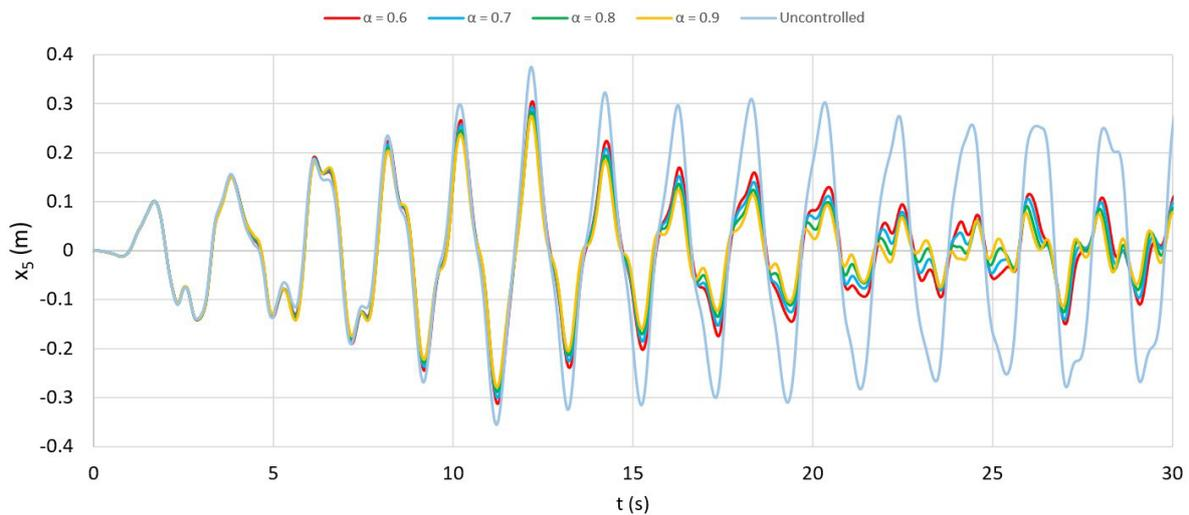
**Figure 17.** Time response of the top of the structure ( $x_5$ ) with the aspect ratio variation for the TLCD with a fixed mass ratio of 5% and designed from the response map.
