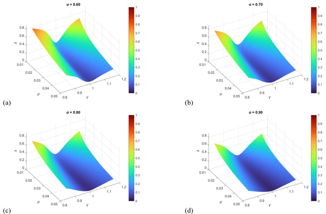
**Figure 7** Surfaces relating the response ratio ( $\lambda$ ) to the parameters of mass ratio ( $\mu$ ) and tuning ratio ( $\gamma$ ), considering different values of aspect ratio: (a)  $\alpha = 0.60$  (b)  $\alpha = 0.70$  (c)  $\alpha = 0.80$  e (d)  $\alpha = 0.90$ .
