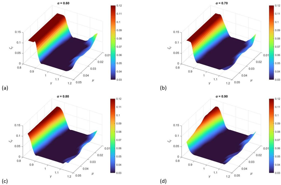
**Figure 9** Surfaces relating the TLCD damping ratio ( $\zeta_f$ ) to the mass ratio ( $\mu$ ) and tuning ratio ( $\gamma$ ) parameters, considering different values of aspect ratio ( $\alpha$ ): (a)  $\alpha = 0.60$  (b)  $\alpha = 0.70$  (c)  $\alpha = 0.80$  e (d)  $\alpha = 0.90$ .
