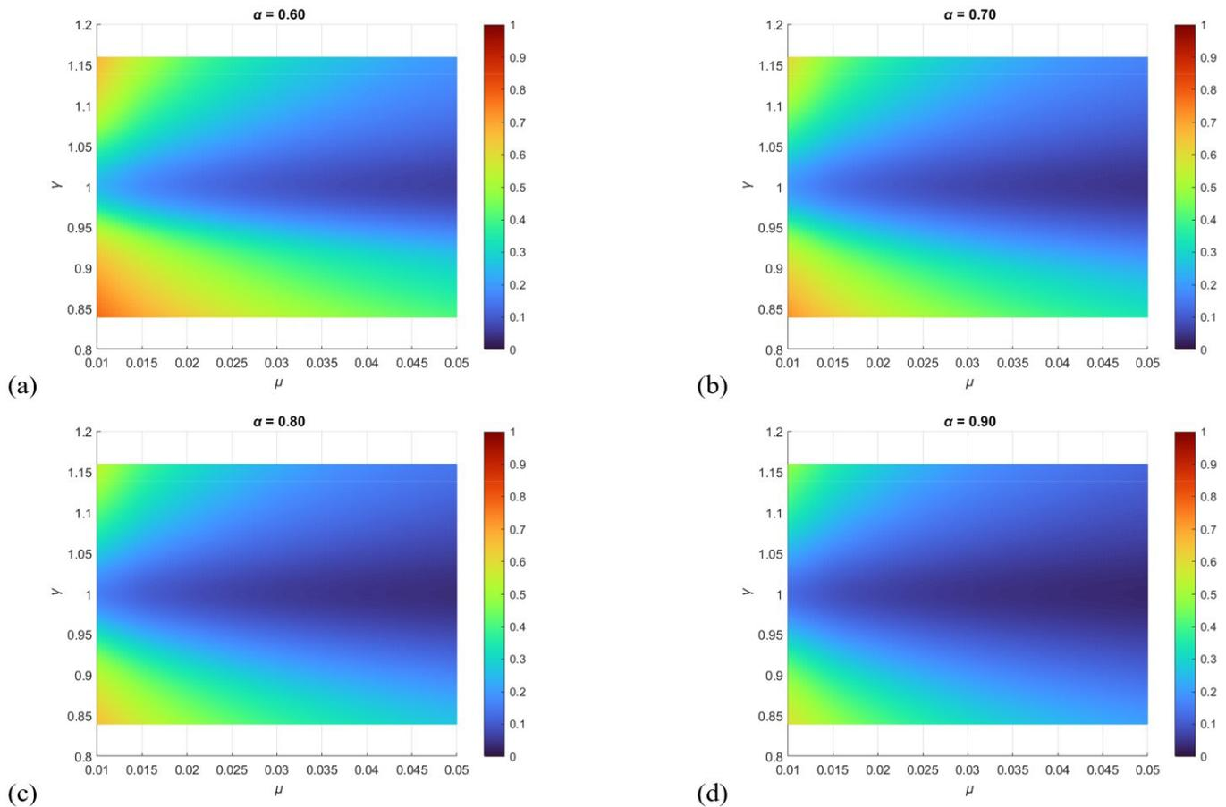
**Figure 8** Colormap relating the response ratio ( $\lambda$ ) to the mass ratio ( $\mu$ ) and the tuning ratio ( $\gamma$ ), considering different values of aspect ratio ( $\alpha$ ): (a)  $\alpha = 0.60$  (b)  $\alpha = 0.70$  (c)  $\alpha = 0.80$  e (d)  $\alpha = 0.90$ .
