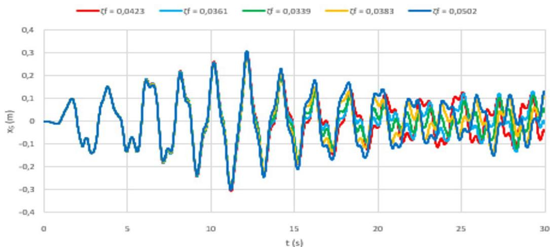
**Figure 18.** Time response of the top of the structure ( $x_5$ ) with the different cases of TLCD damping ratio as presented in Table 3.
