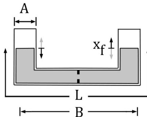
Figure 2: Configuration of the tuned liquid column damper (TLCD).
