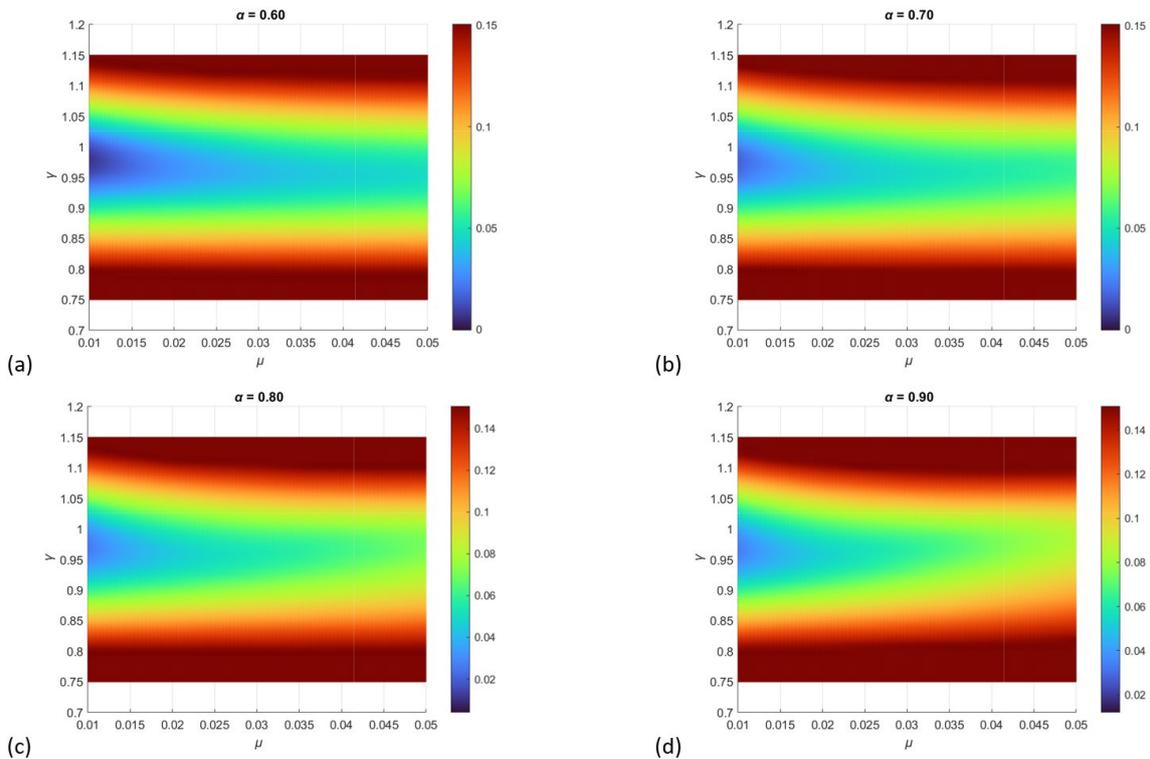
**Figure 15** Colormap relating the TLCD damping ratio ( $\zeta_f$ ) to the mass ratio ( $\mu$ ) and tuning ratio ( $\gamma$ ) parameters, considering different values of aspect ratio ( $\alpha$ ): (a)  $\alpha = 0.60$  (b)  $\alpha = 0.70$  (c)  $\alpha = 0.80$  e (d)  $\alpha = 0.90$ .
