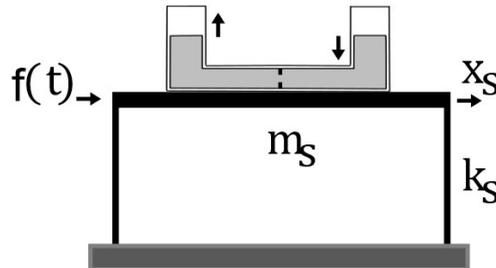
Figure 3: Structure with TLCD attached.
