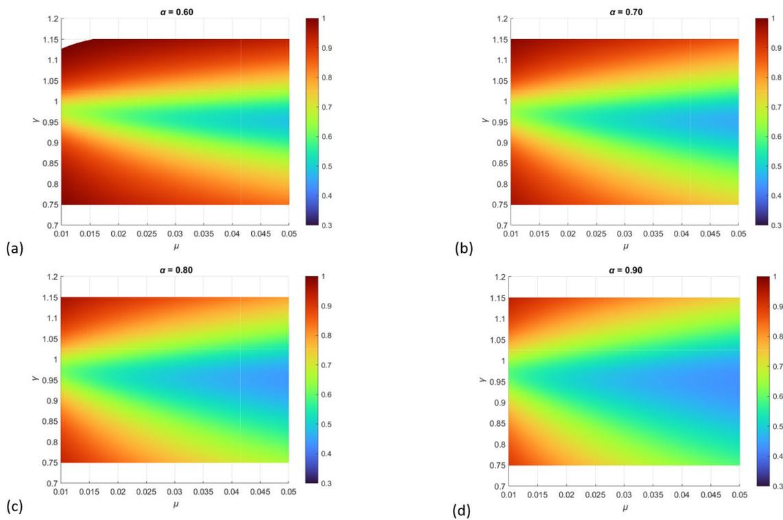
**Figure 13** Colormap relating the structure response ratio ( $\lambda$ ) for the El Centro earthquake to the parameters of mass ratio ( $\mu$ ) and tuning ratio ( $\gamma$ ), considering different values of aspect ratio ( $\alpha$ ): (a)  $\alpha = 0.60$  (b)  $\alpha = 0.70$  (c)  $\alpha = 0.80$  e (d)  $\alpha = 0.90$ .
