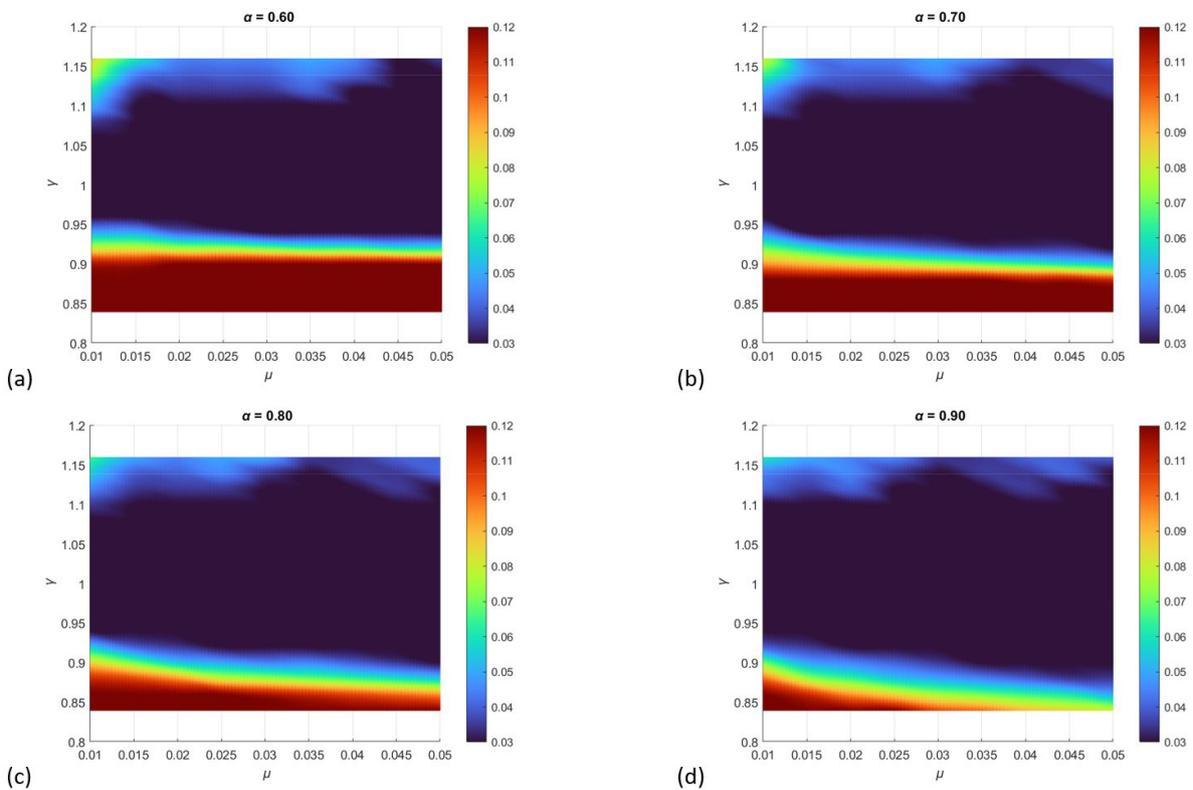
**Figure 10** Colormap relating the response ratio ( $\zeta_r$ ) to the mass ratio ( $\mu$ ) and the tuning ratio ( $\gamma$ ), considering different values of aspect ratio ( $\alpha$ ): (a)  $\alpha = 0.60$  (b)  $\alpha = 0.70$  (c)  $\alpha = 0.80$  e (d)  $\alpha = 0.90$ .
