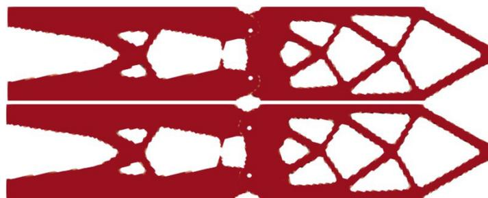
**Figure 8** Cantilever with two domains (Sequential Optimization): Optimized Side Views
