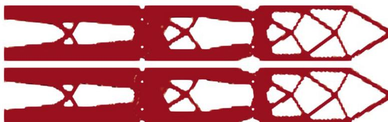
**Figure 20** Cantilever with three domains (Normal Optimization): Optimized Side Views
