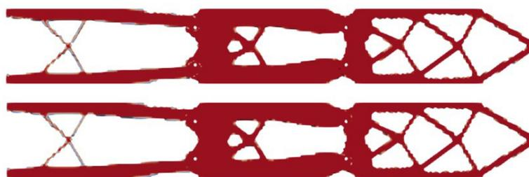
**Figure 24** Cantilever with three domains (Sequential Optimization): Optimized Side Views - Volume of 30% for Component 1 and 50% for a Components 2 and 3
