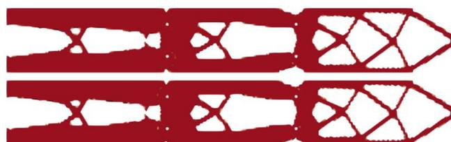
**Figure 22** Cantilever with three domains (Sequential Optimization): Optimized Side Views
