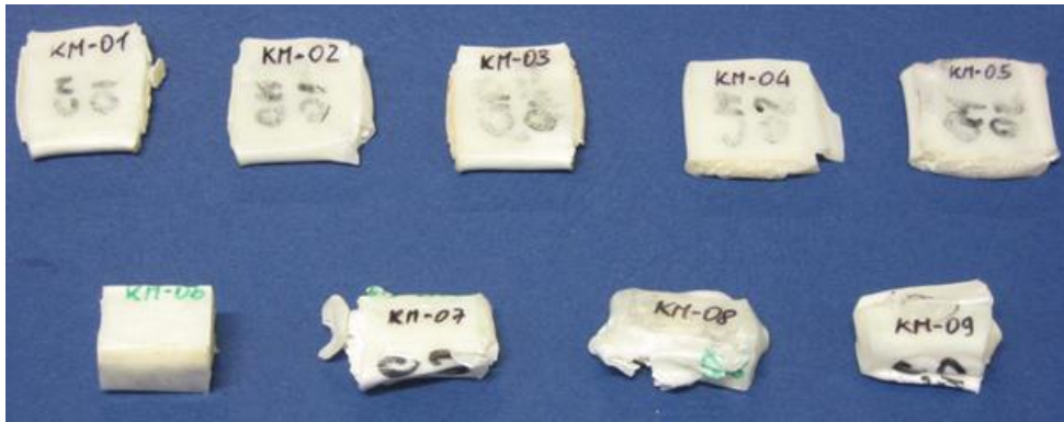
Figure 21 Microcellular foam samples loaded on the largest (KM-01 to KM-06) and smallest side (KM-07 to KM-09).
