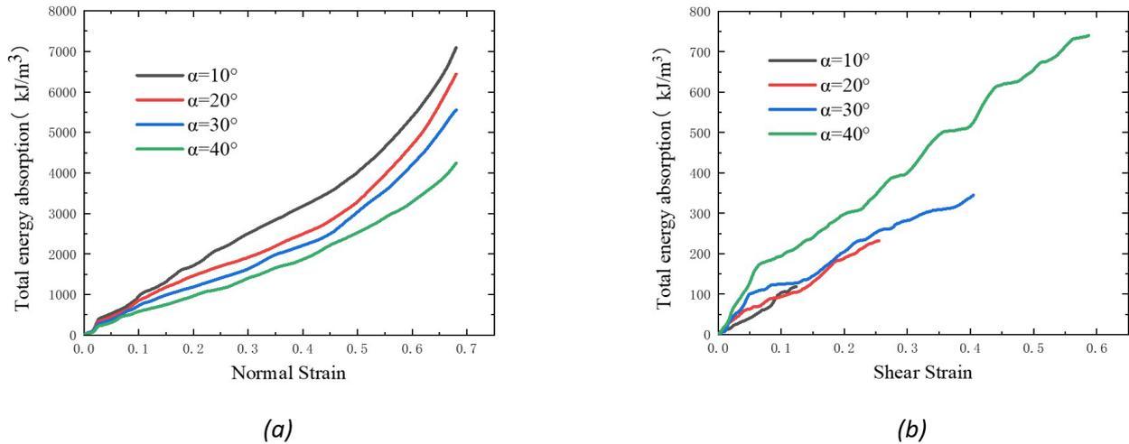
Figure 30. Total energy absorption of star-shaped auxetic honeycomb ( $v = 40$  m/s): (a) Normal direction; (b) Shear direction.
