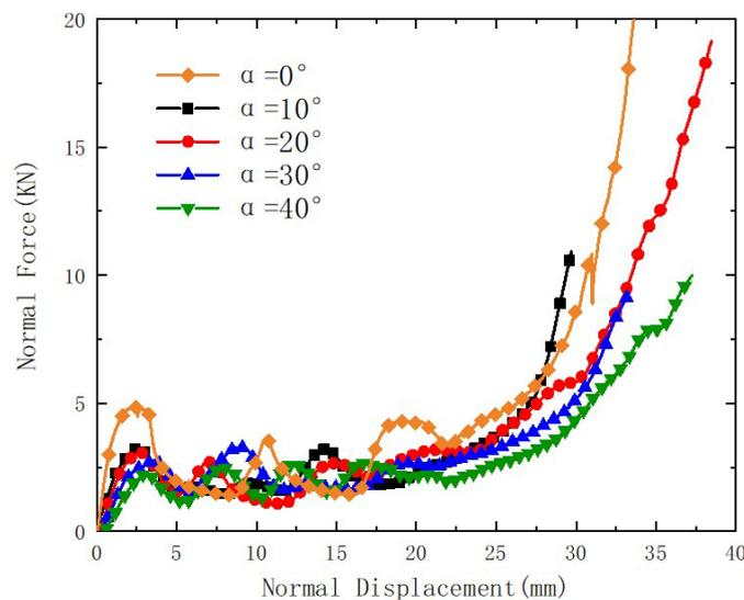
Figure 6. Normal load-displacement curve of star-shaped auxetic honeycomb under complex loading.
