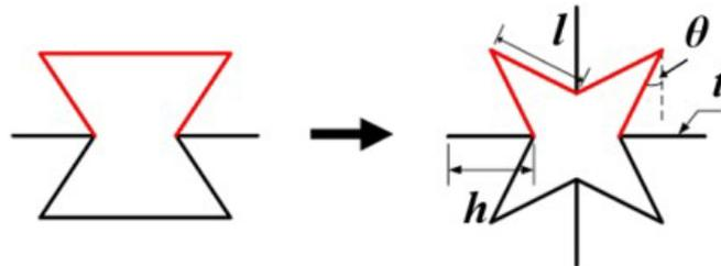
Figure 1. Star-shaped auxetic honeycomb and its geometric parameters.
