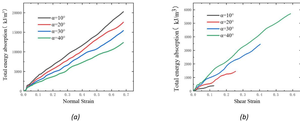
Figure 31. Total energy absorption of star-shaped auxetic honeycomb ( $v = 120$  m/s): (a) Normal direction; (b) Shear direction.
