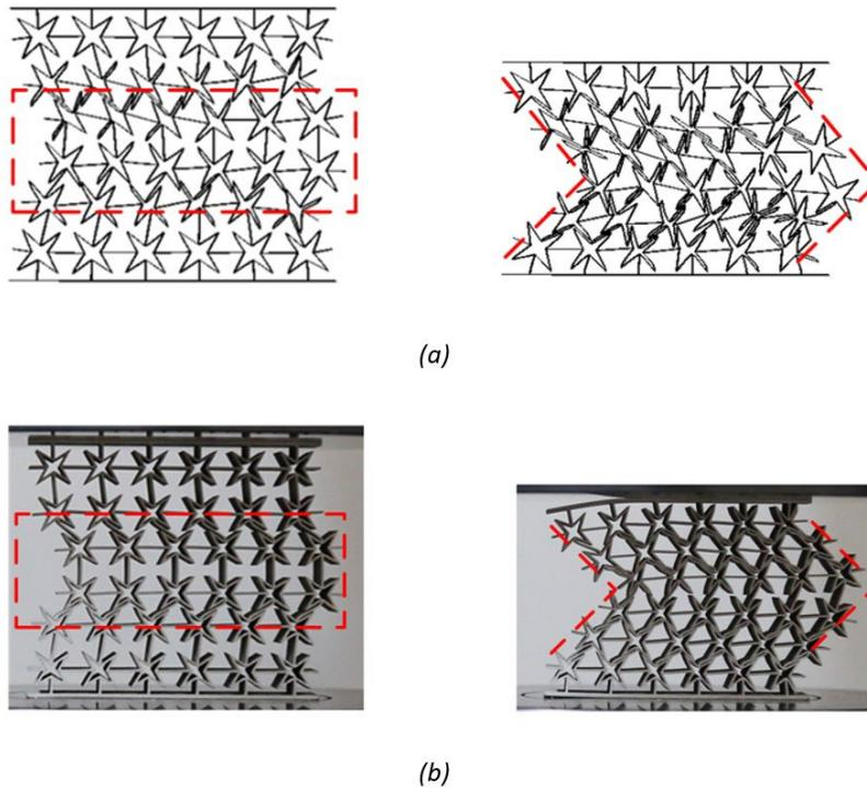
Figure 14. Comparison of complex loading experimental and simulation deformation mode results( $\alpha = 0^\circ$ ): (a) Simulation ; (b) Experiment
