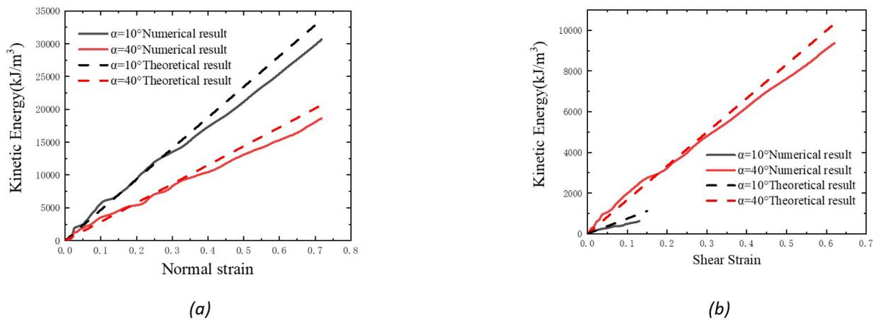
Figure 34. Comparison between simulation results and theoretical values of kinetic energy of star-shaped auxetic honeycomb under high-speed loading ( $v = 150$  m/s): (a) Normal; (b) Shear
