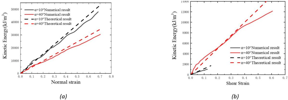
**Figure 35.** Comparison between simulation results and theoretical values of kinetic energy of star-shaped auxetic honeycomb under high-speed loading ( $v = 200$  m/s): (a) Normal; (b) Shear
