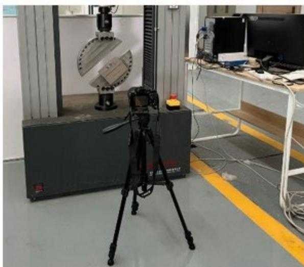
**Figure 4.** Combined compression–shear loading system.
