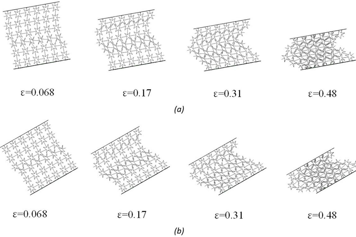
**Figure 16.** Deformation mode of star-shaped auxetic honeycomb under combined compression and shear loading ( $v = 0.1 \text{ m/s}$ ): (a)  $\alpha = 10^\circ$ ; (b)  $\alpha = 30^\circ$
