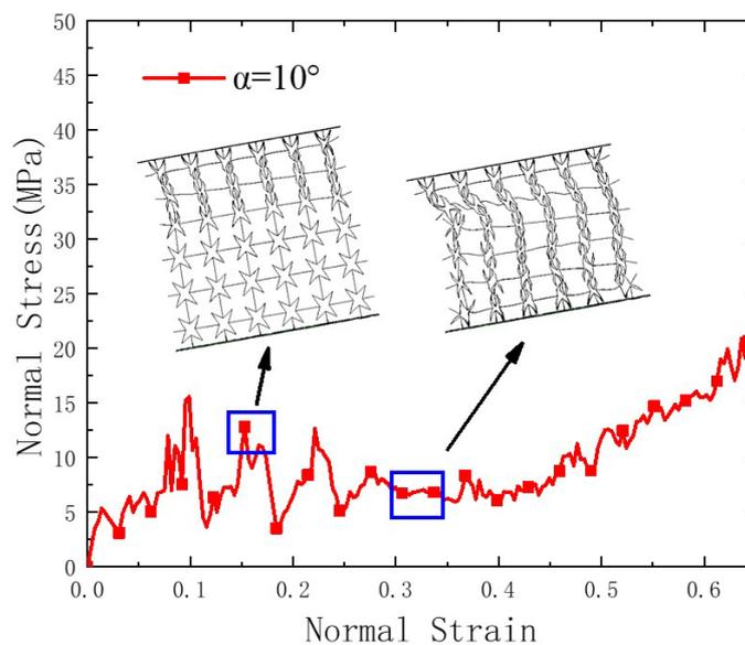
**Figure 24.** Stress–strain curve of star-shaped auxetic honeycomb under combined compression–shear loading ( $\alpha = 10^\circ$ ,  $v = 40$  m/s).
