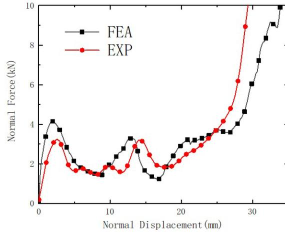
Figure 12. Comparison of normal load displacement simulation and experimental results under combined loading( $\alpha = 10^\circ$ ).
