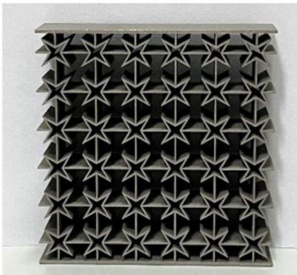
**Figure 3.** Star-shaped auxetic honeycomb specimen.
