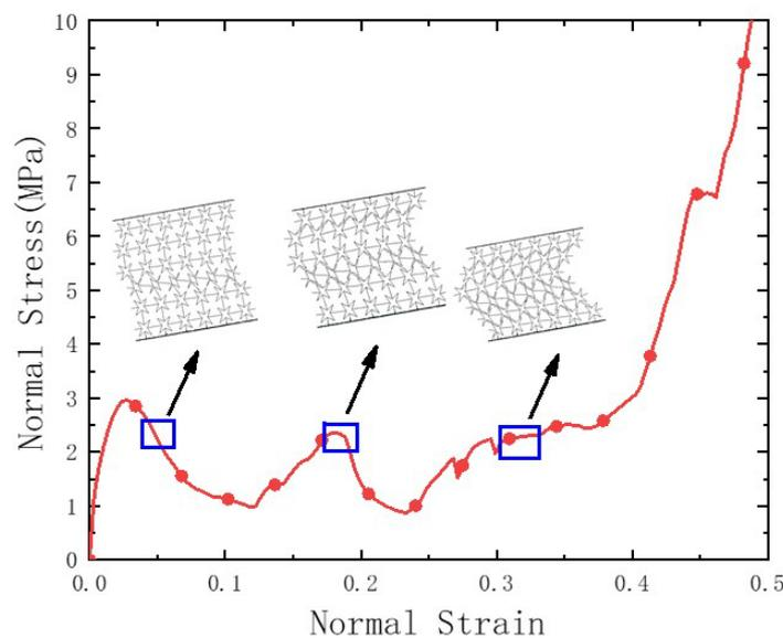
**Figure 23.** Stress–strain curve of star-shaped auxetic honeycomb under combined compression–shear loading ( $\alpha = 10^\circ$ ,  $v = 0.1$  m/s).
