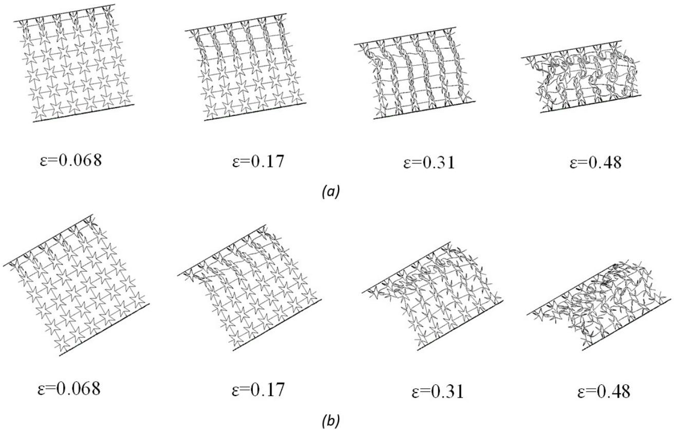
**Figure 17.** Deformation mode of star-shaped auxetic honeycomb under combined compression and shear loading ( $v = 40 \text{ m/s}$ ): (a)  $\alpha = 10^\circ$ ; (b)  $\alpha = 30^\circ$
