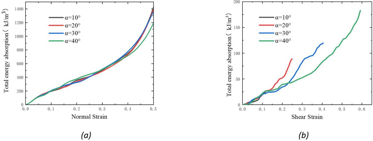
Figure 29. Total energy absorption of star-shaped auxetic honeycomb ( $v = 0.1$  m/s): (a) Normal direction; (b) Shear direction.
