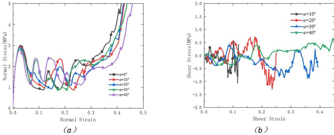
**Figure 20.** Stress–strain curves of star-shaped auxetic honeycomb under low-speed ( $v = 0.1$  m/s) combined compression–shear loading: (a) Normal direction; (b) Shear direction.
