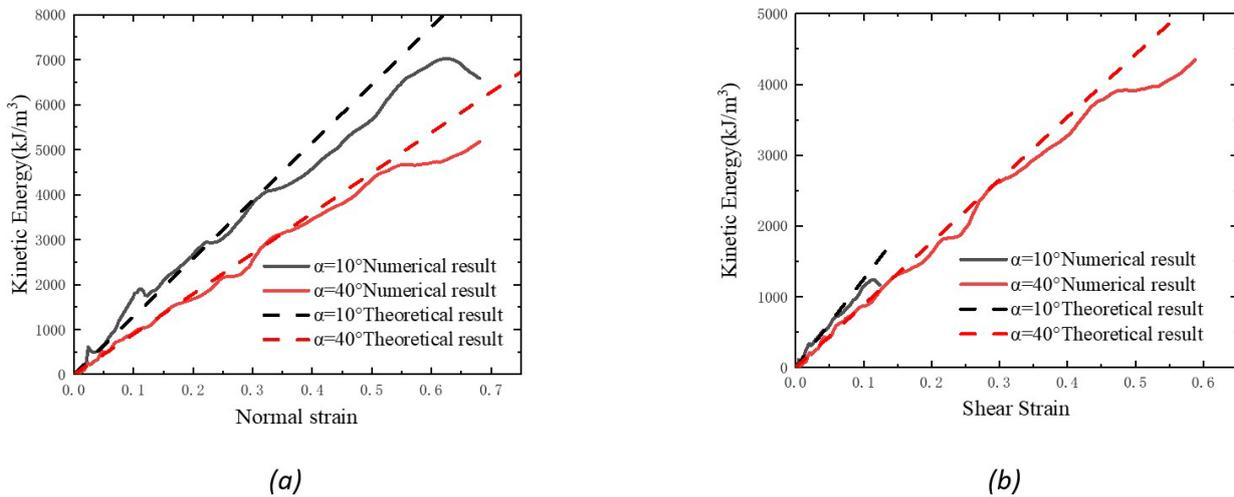
Figure 33. Comparison between simulation results and theoretical values of kinetic energy of star-shaped auxetic honeycomb under high-speed loading ( $v = 120$  m/s): (a) Normal; (b) Shear
