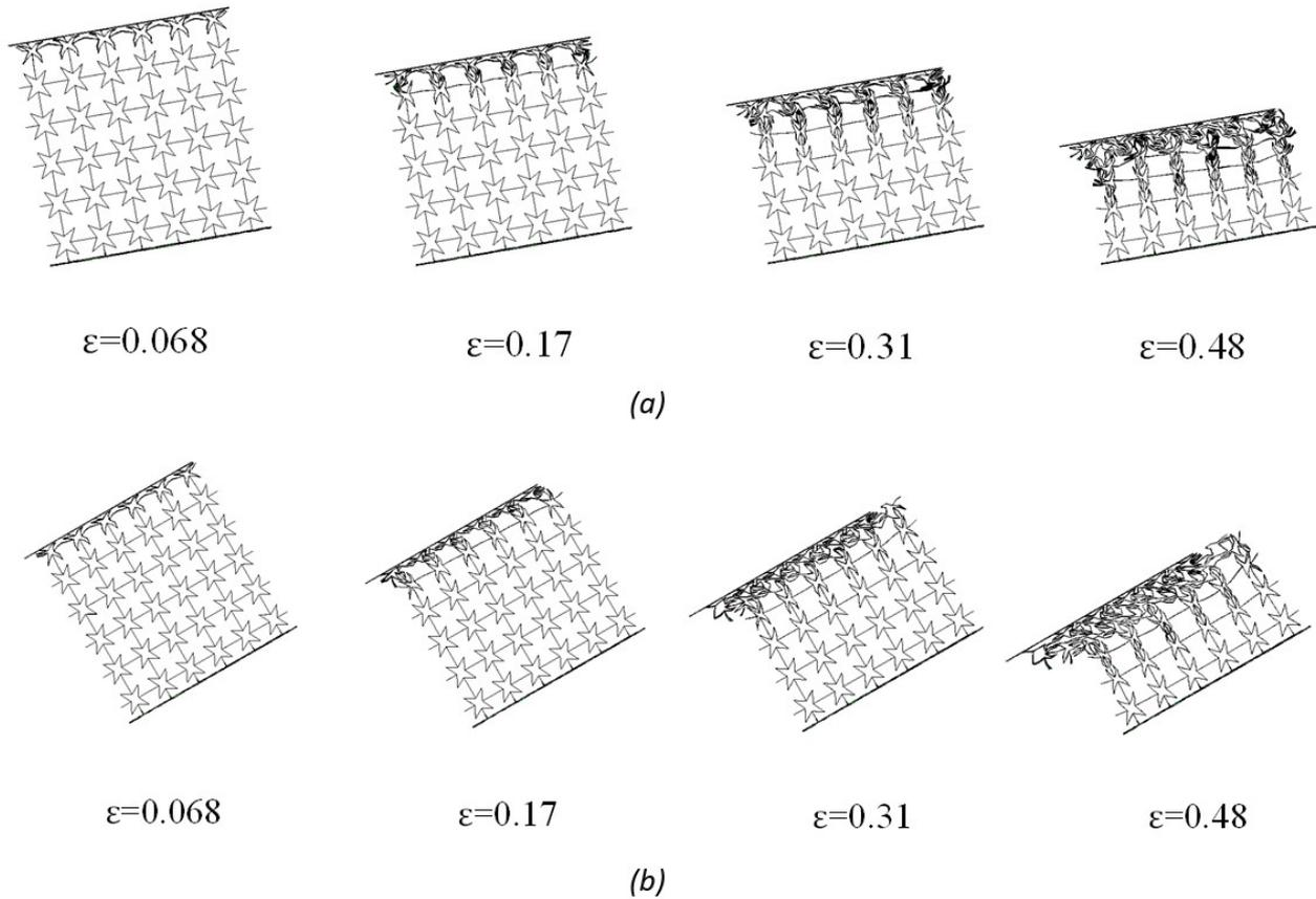
**Figure 18.** Deformation mode of star-shaped auxetic honeycomb under combined compression and shear loading ( $v = 120\text{m/s}$ ): (a)  $\alpha=10^\circ$ ; (b)  $\alpha=30^\circ$
