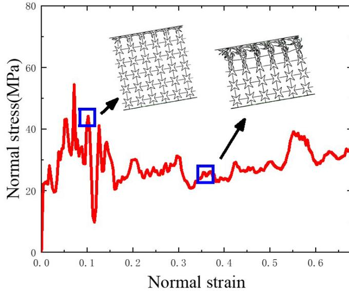
Figure 25. Stress–strain curve of star-shaped auxetic honeycomb under combined compression–shear loading( $\alpha = 10^\circ$ ,  $v = 120$  m/s).
