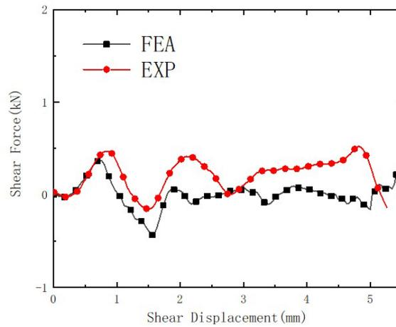
Figure 13. Comparison of shear load displacement simulation and experimental results under combined Loading( $\alpha = 10^\circ$ ).
