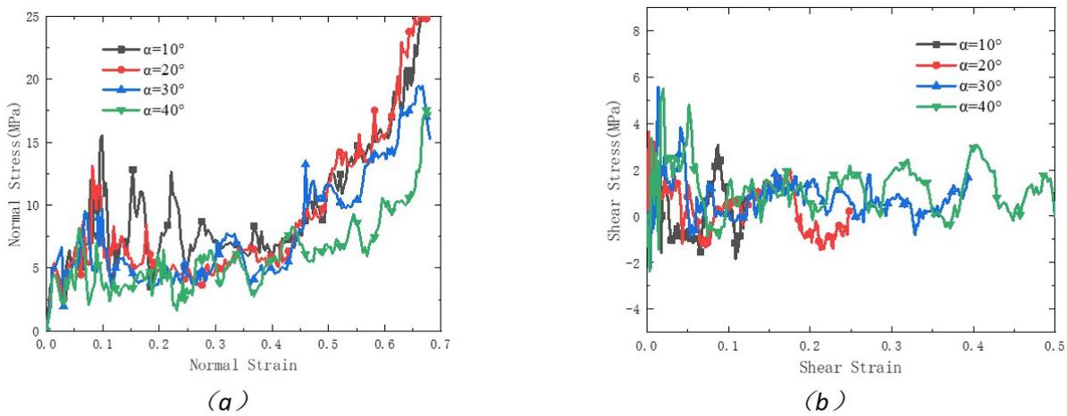
**Figure 21.** Stress–strain curve of star-shaped auxetic honeycomb under medium-speed ( $v = 40$  m/s) combined compression–shear loading: (a) Normal direction; (b) Shear direction.
