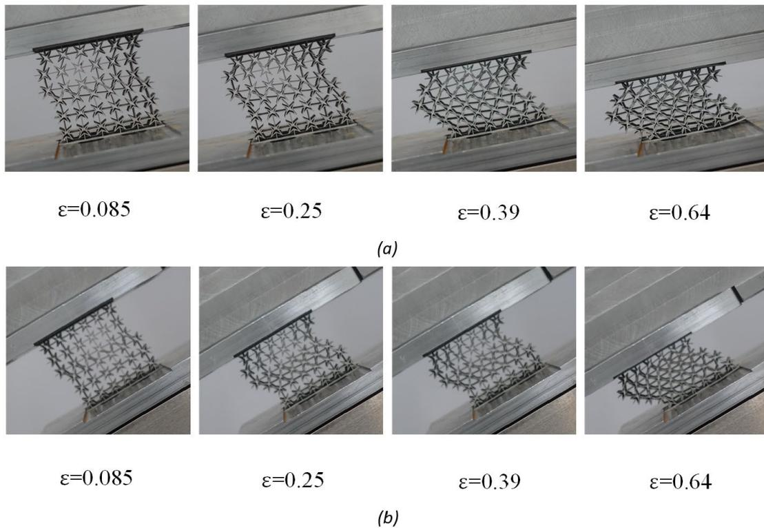
Figure 8. Deformation mode of star-shaped auxetic honeycomb specimen under complex loading: (a)  $\alpha=10^\circ$ ; (b)  $\alpha=30^\circ$
