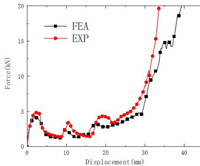
Figure 11. Comparison between numerical and experimental results of uniaxial compression load displacement( $\alpha = 0^\circ$ ).
