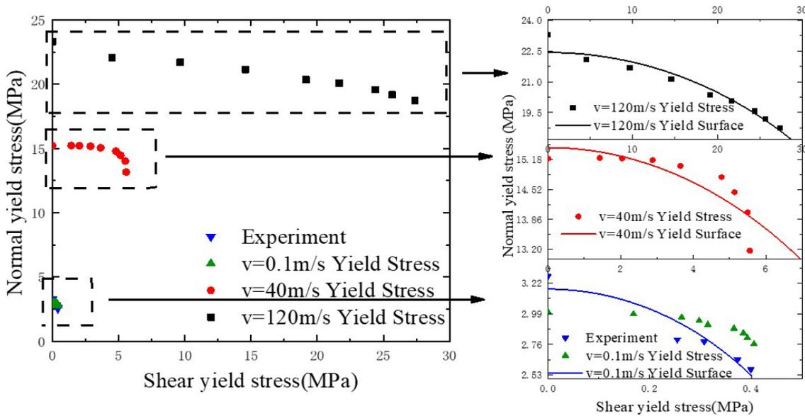
Figure 28. Yield surface of star-shaped auxetic honeycomb under combined compression–shear loadings.
