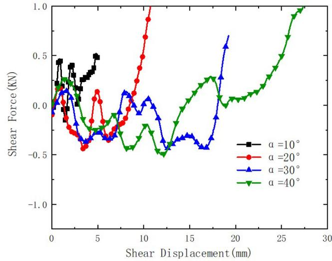
Figure 7. Shear load-displacement curve of star-shaped auxetic honeycomb under complex loading.
