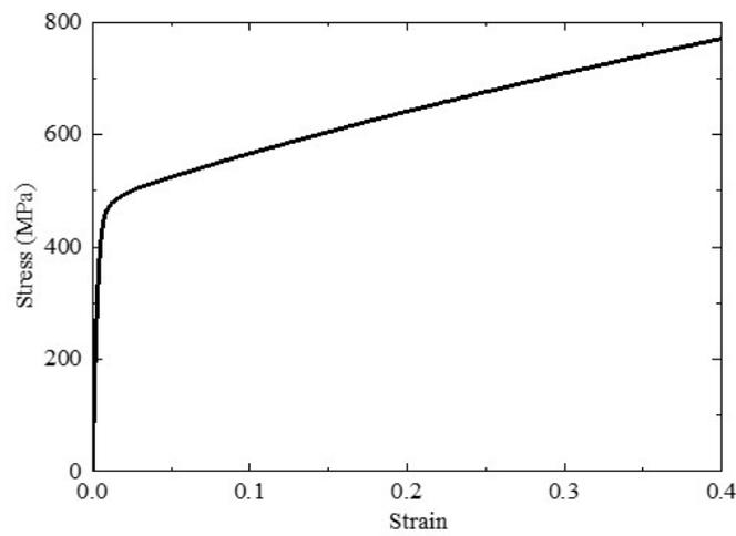
Figure 10. Stress-strain curve of 316L
