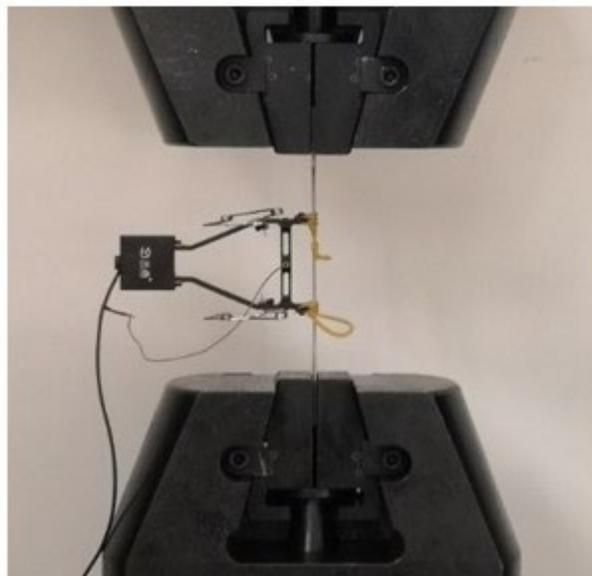
Figure 2. Tensile experiment of 316L stainless steel substrate.
