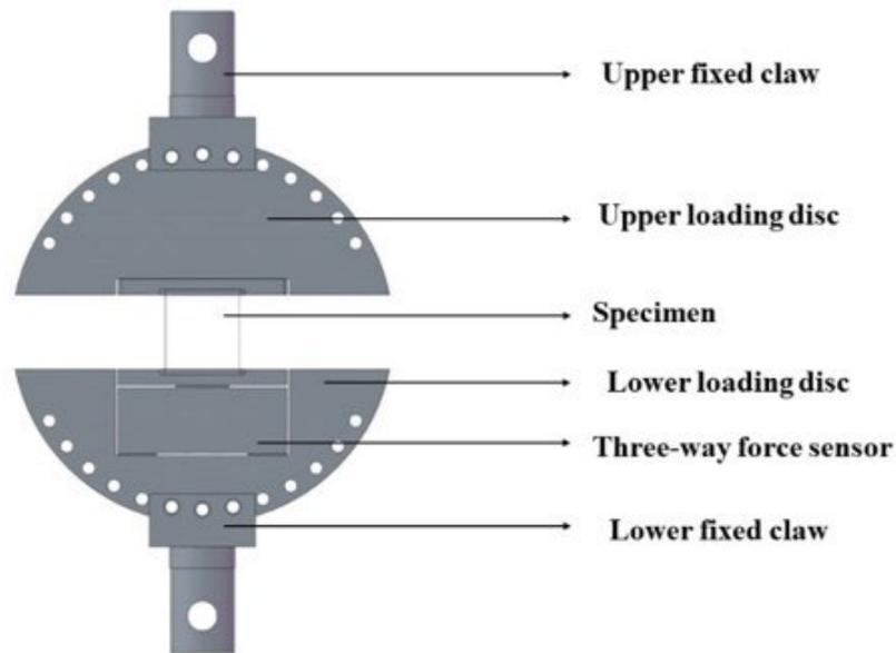
Figure 5. Variable-angle loading fixture.
