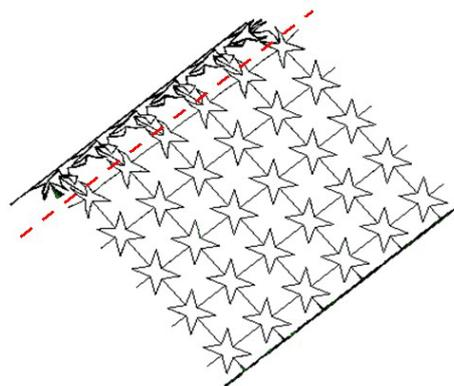
Figure 32. Plastic shock wave of star-shaped auxetic honeycomb.
