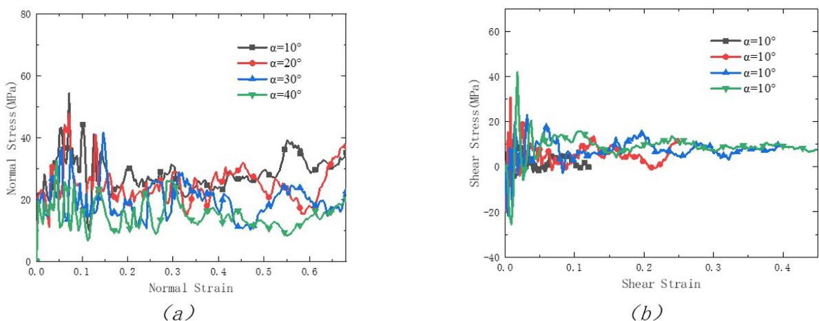
**Figure 22.** Stress–strain curve of star-shaped auxetic honeycomb under high-speed ( $v = 120$  m/s) combined compression–shear loading: (a) Normal direction; (b) Shear direction.
