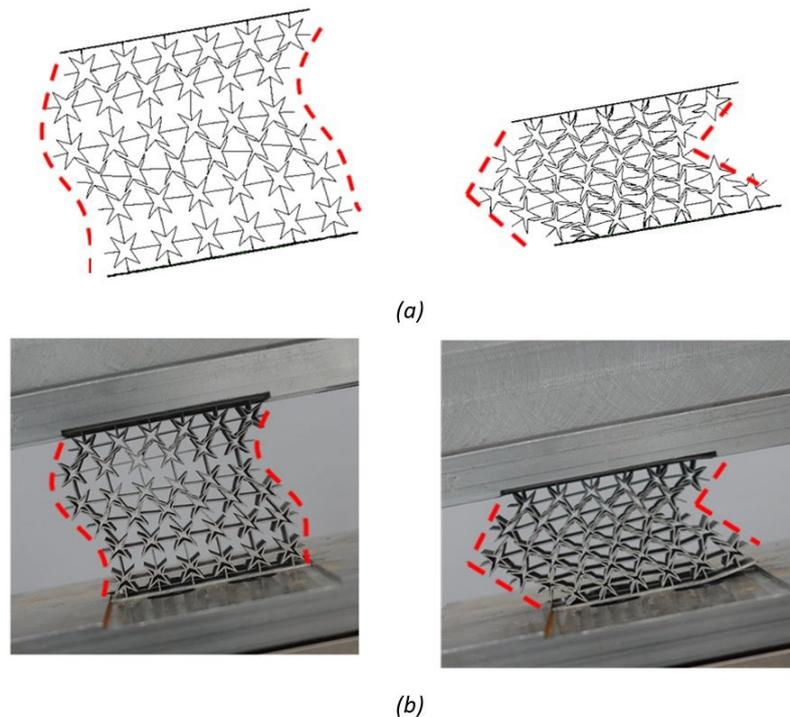
**Figure 15.** Comparison of complex loading experimental and simulation deformation mode results( $\alpha = 10^\circ$ ): (a) Simulation ; (b) Experiment
