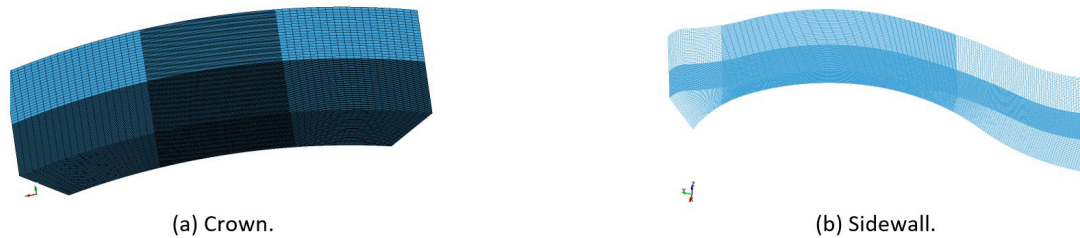
Figure 8 Mesh of the crown and sidewall.
