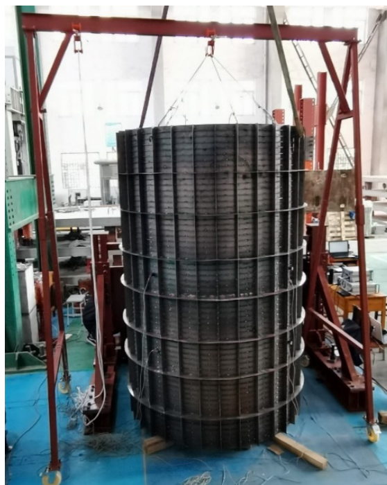
Fig 3. Model of iron stiffened cylindrical shell.
