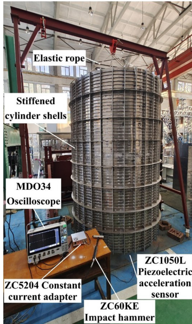
Fig 4. Suspension and testing system for free vibration test.
