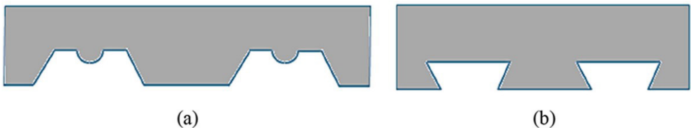
Figure 1 Shape of profile deck (a) Trapezoidal deck (b) Re-entrant profile
