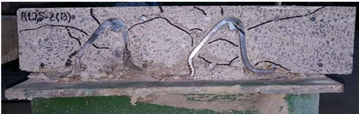
Figure 15 Section on the TTR connectors alignment of specimen after the push-out test performed by Barbosa (2016)
