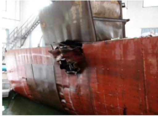
**Figure 13** Explosion test on ships with multiple compartments.
