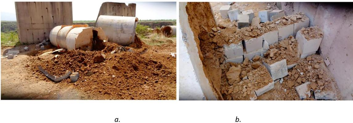
**Figure 5** Penetration effect of the  $\phi 148$  mm shaped charge jet on the asphalt/soil/concrete composite target.
