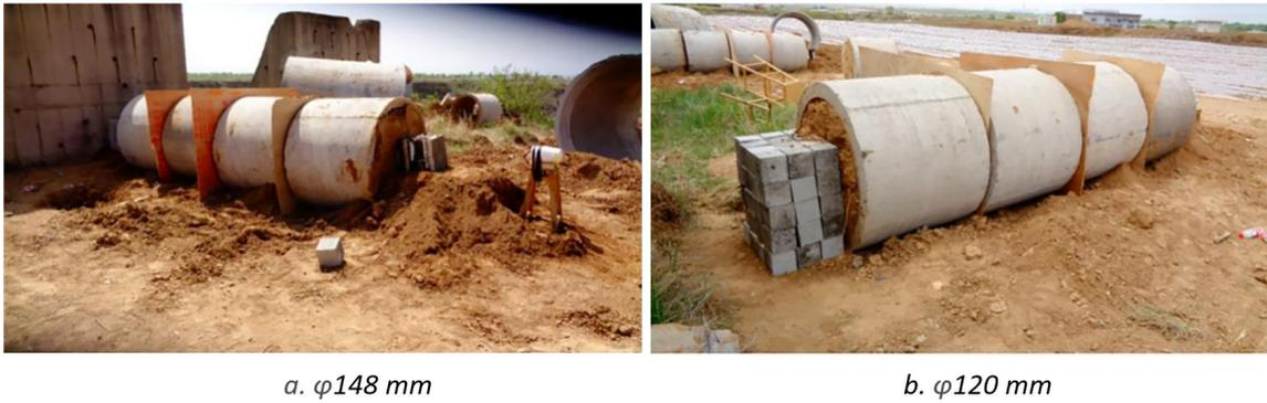
**Figure 4** Experimental device for the penetration of shaped charges into asphalt/soil/concrete composite targets.
