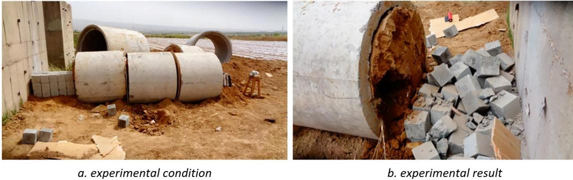
Figure 17 Experimental condition and result with the  $\phi 120$  mm shaped charge.
