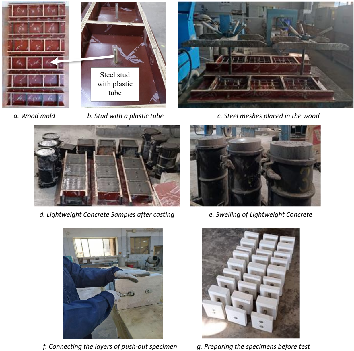
Figure 3 The fabrication process of PLCSS.
