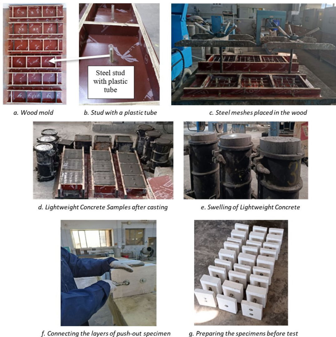
Figure 3 The fabrication process of PLCSS.
