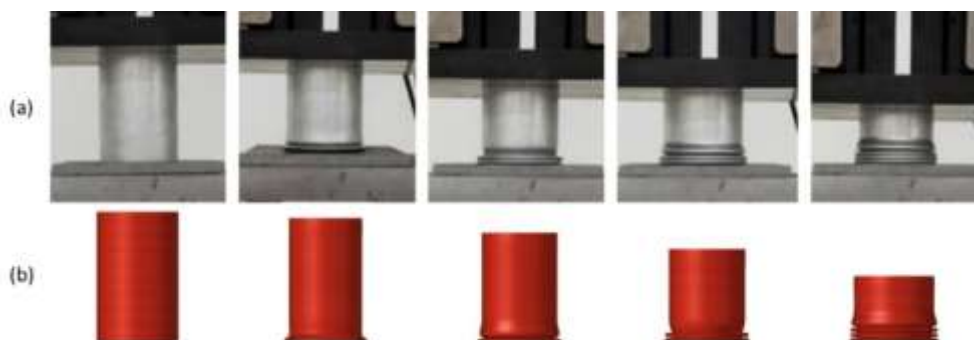
Figure 7 Comparison of deformation modes (a) experimental test (Altin et al., 2017) (b) FE model.
