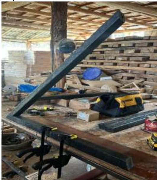
Figure 16 Connection of Elements to Form the Triangles of the Frequency 3 Dome.
