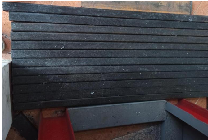
Figure 15 Result of the Polypropylene Extrusion, Elements with 50 × 50 mm Section and 2.15 m Length.
