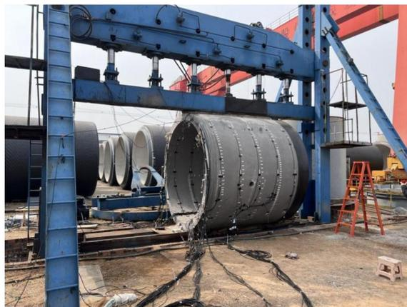
**Figure 4** Three-edge bearing test method device.
