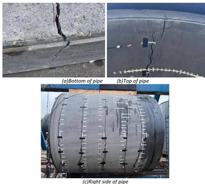
**Figure 11** Pipe cracking and damage
