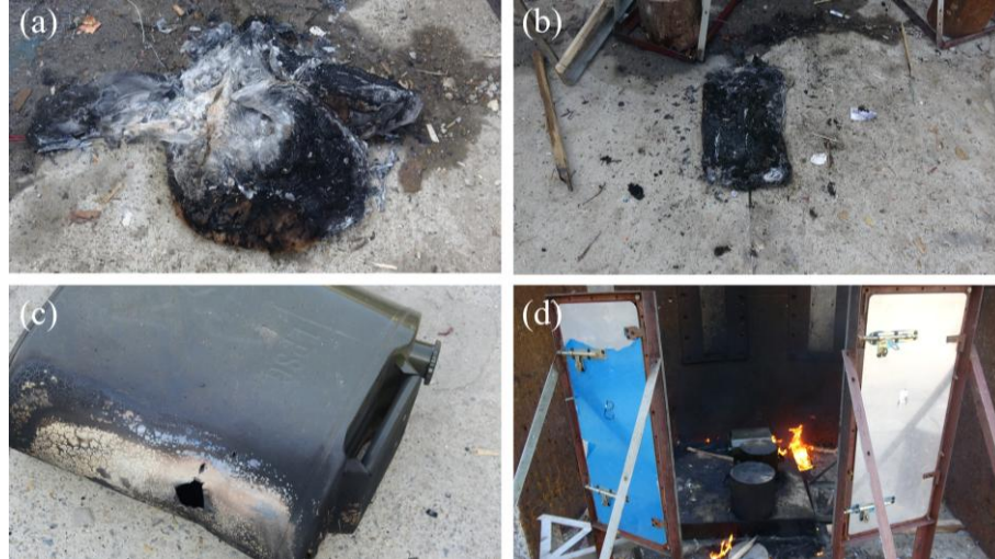
Figure 9 Damage of the quilt and oil tank.
