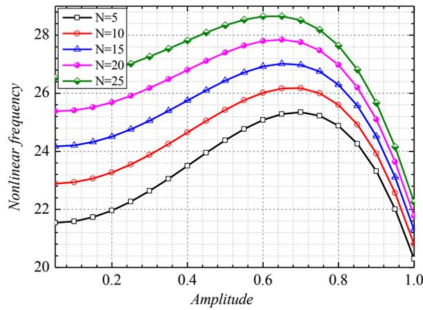
Figure 6 Effect of  $N$  parameter on nonlinear frequency of electrostatically microbeam base on amplitude
