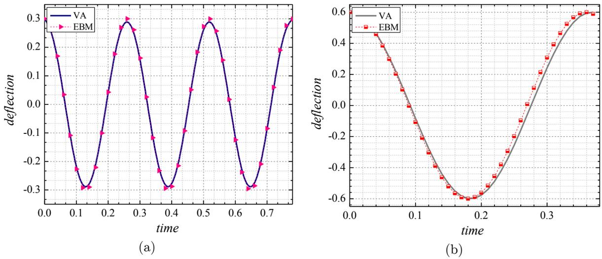
Figure 2 Comparison of variational approach solution of deflection with the EBM solution based on time for cases (a):  $N = 10, a = 24, V = 10, A = 0.3$  (b):  $N = 10, a = 24, V = 20, A = 0.6$
