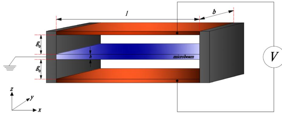
Figure 1 Schematics of a double-sided driven clamped-clamped microbeam-based electromechanical resonator
