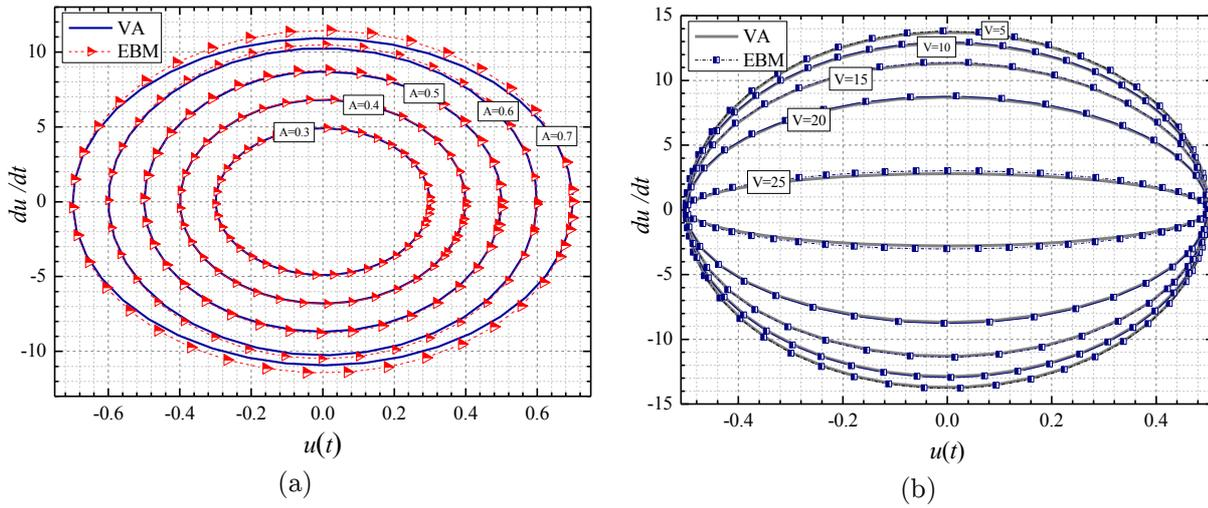
Figure 4 (a): Effect of amplitude on the phase plan of the problem for  $N = 10$ ,  $a = 24$ ,  $V = 10$
