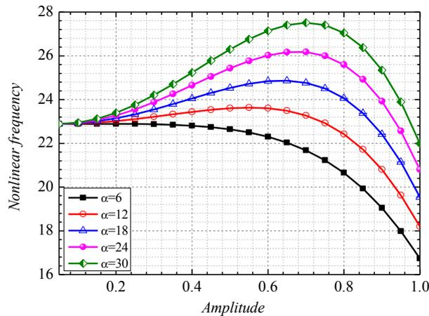
Figure 7 Effect of  $\alpha$  parameter on nonlinear frequency of electrostatically microbeam base on amplitude
