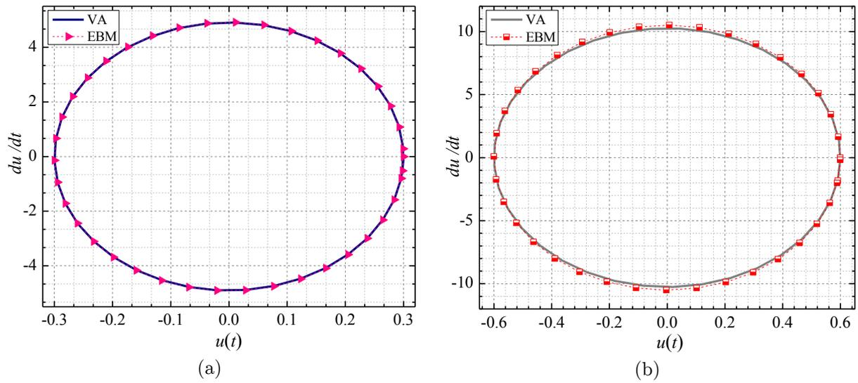
Figure 3 Comparison of variational approach solution of phase plan with the EBM solution for cases (a):  $N = 10, a = 24, V = 10, A = 0.3$  (b):  $N = 10, a = 24, V = 20, A = 0.6$
