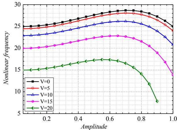
Figure 5 Effect of V parameter on nonlinear frequency of electrostatically microbeam base on amplitude
