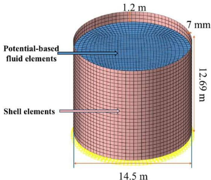
**Figure 5** FEM of the Anchored Storage Tank
