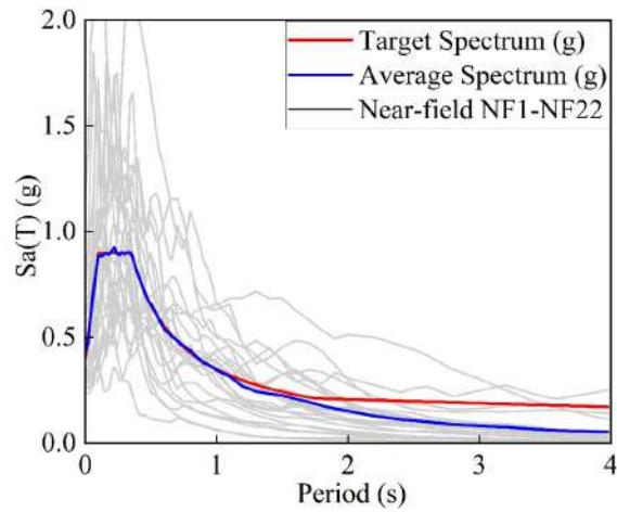
**Figure 2** Comparison of Near-Field Motion Response Spectrum and Its Average with Target Response Spectrum
