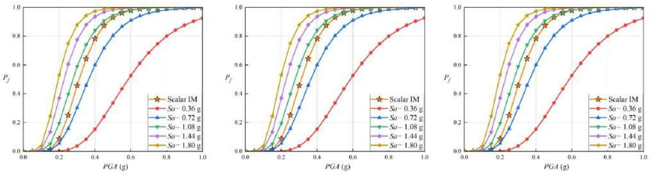
(a) Comparison of damage probability between scalar and vector values of  $h_v$
