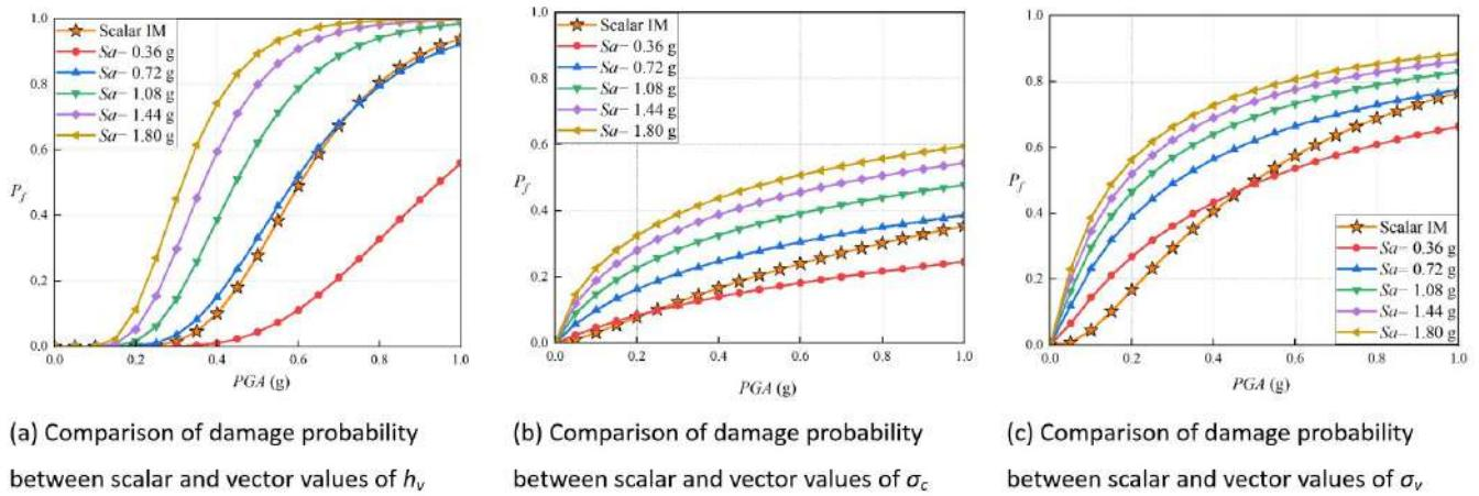
**Figure 17** Comparison of vector-valued vulnerability surfaces and scalar-valued vulnerability curves for three failure modes under DS5
