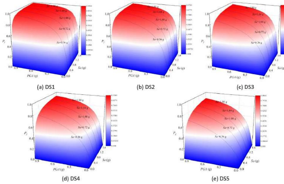
**Figure 12** Vulnerability surfaces of  $\sigma_v$  under different damage states
