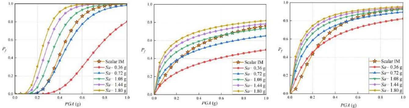
(a) Comparison of damage probability between scalar and vector values of  $h_v$
