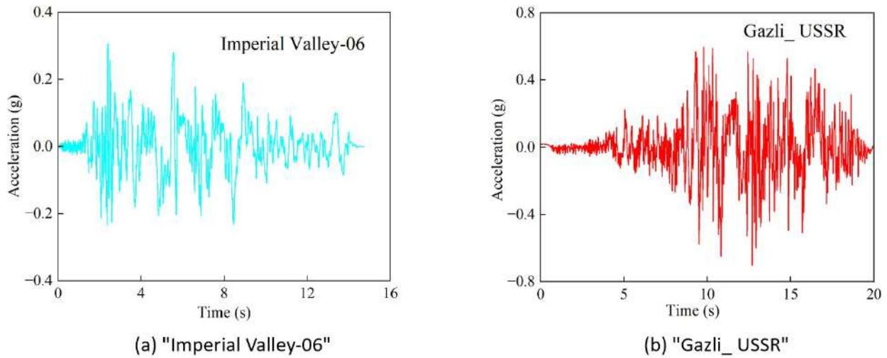
**Figure 3** Selected partial seismic acceleration curve records
