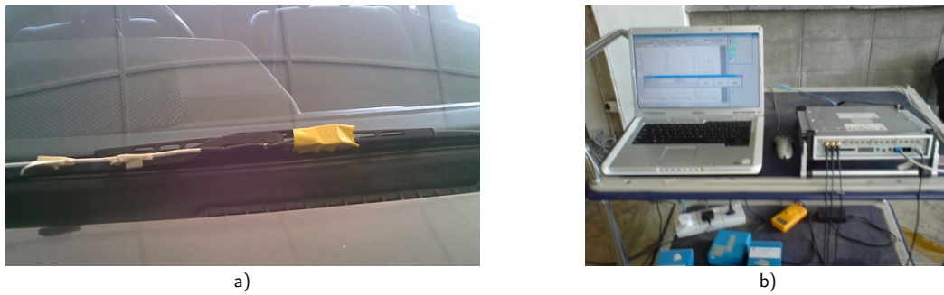
Figure 2 (a) Kistler type 8794A500 tri-axial accelerometer; (b) PAK MK II Muller BBM analyzer.
