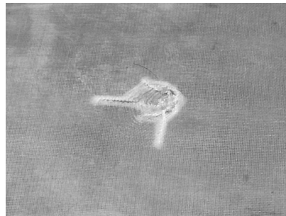
Figure 8: 3 layer Glass Fabric/Epoxy laminate showing the formation of concentric ring around the impact region
