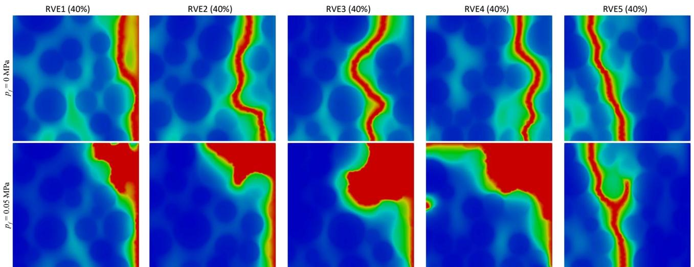
**Figure 6** Phase-field contour plot for aggregate volume fraction of 40% for five RVEs with random particle distributions: without pressure load (first row) and with pressure load  $p_f = 0.05$  MPa (second row).
