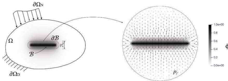
**Figure 1** Phase-field model: a solid body with a phase-field crack with pressure load.
