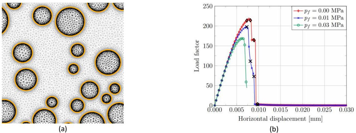
**Figure 9** RVE with mortar, 0.35 aggregate fraction, and ITZ: (a) Finite element mesh; (b) Equilibrium trajectory for different pressure load values (black markers indicate the selected stages along the equilibrium paths for which the phase-field contours are shown in Fig. 10).
