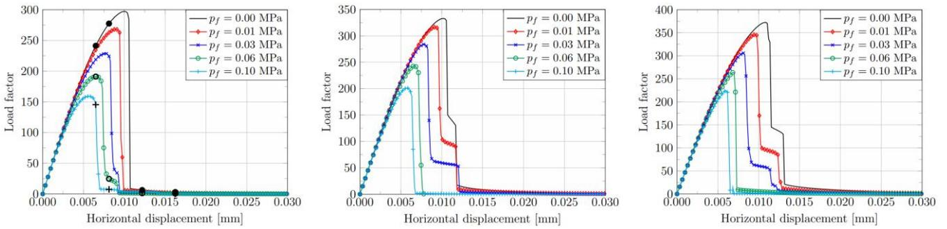
**Figure 7** Equilibrium trajectory for different pressure load values: Aggregate volume fraction of 30% (first graph), aggregate volume fraction of 35% (second graph), aggregate volume fraction of 40% (third graph). Black markers in the first graph indicate the selected stages along the equilibrium paths for which the phase-field contours are shown in Fig. 8.
