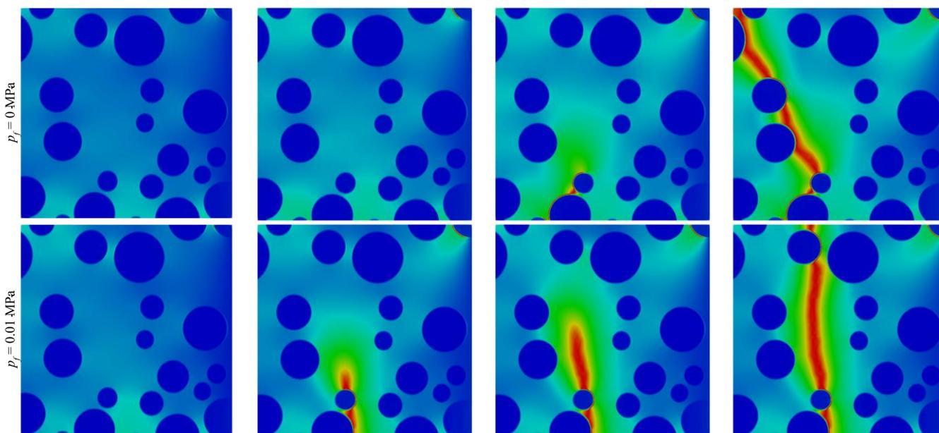
**Figure 10** Phase-field contour plot for aggregate volume fraction of 35% with ITZ: Step 45 (first column), step 50 (second column), step 55 (third column), step 60 (fourth column).
