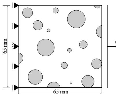
**Figure 3** Problem setting: tensile test on heterogeneous RVEs.
