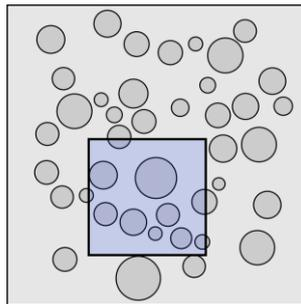
**Figure 2** Initial larger domain containing the distributed aggregates, from which the RVE with the specified dimensions is extracted.
