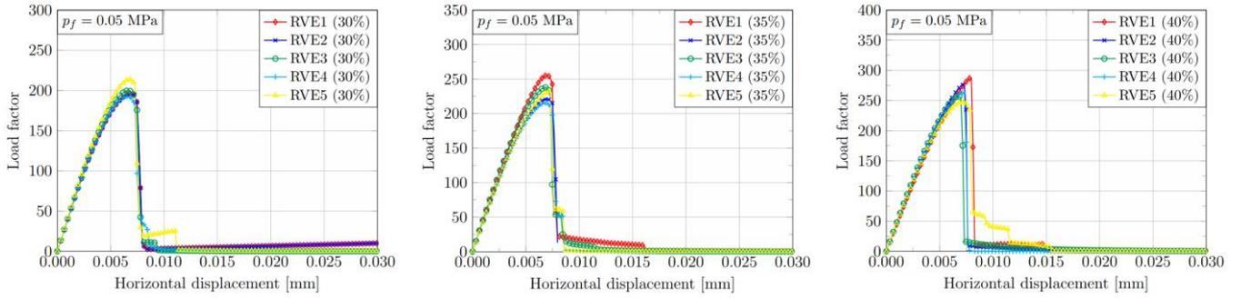
**Figure 5** Equilibrium trajectory for RVEs with different particle distributions without pressure load (first row) and with pressure load  $p_f = 0.05$  MPa (second row). RVEs with the same index (RVE $i$ , with  $i = 1-5$ ) do not represent the same microstructure across different aggregate fractions.
