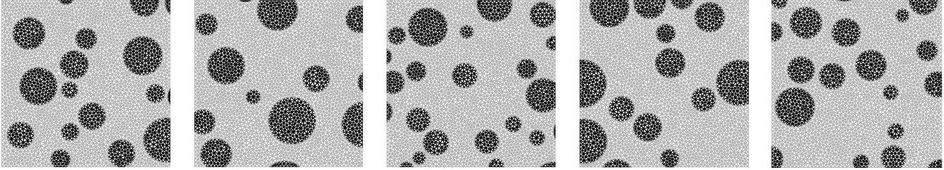
**Figure 4** Finite element meshes for RVEs with aggregate volume fraction of 30% and different particle distributions.
