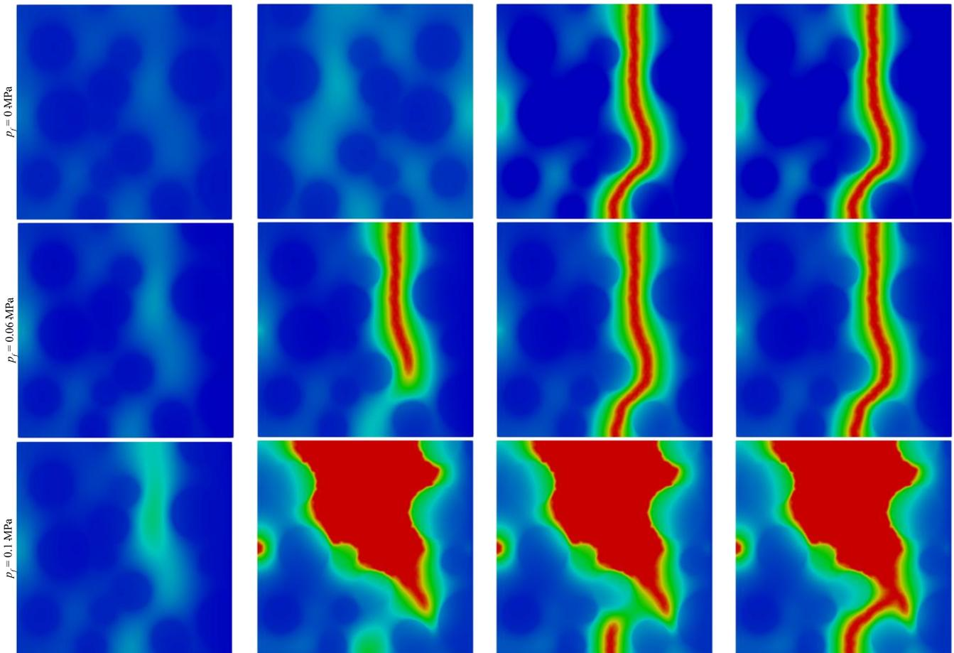
**Figure 8** Phase-field contour plot for aggregate volume fraction of 30%: Step 40 (first column), step 50 (second column), step 75 (third column), step 100 (fourth column).
