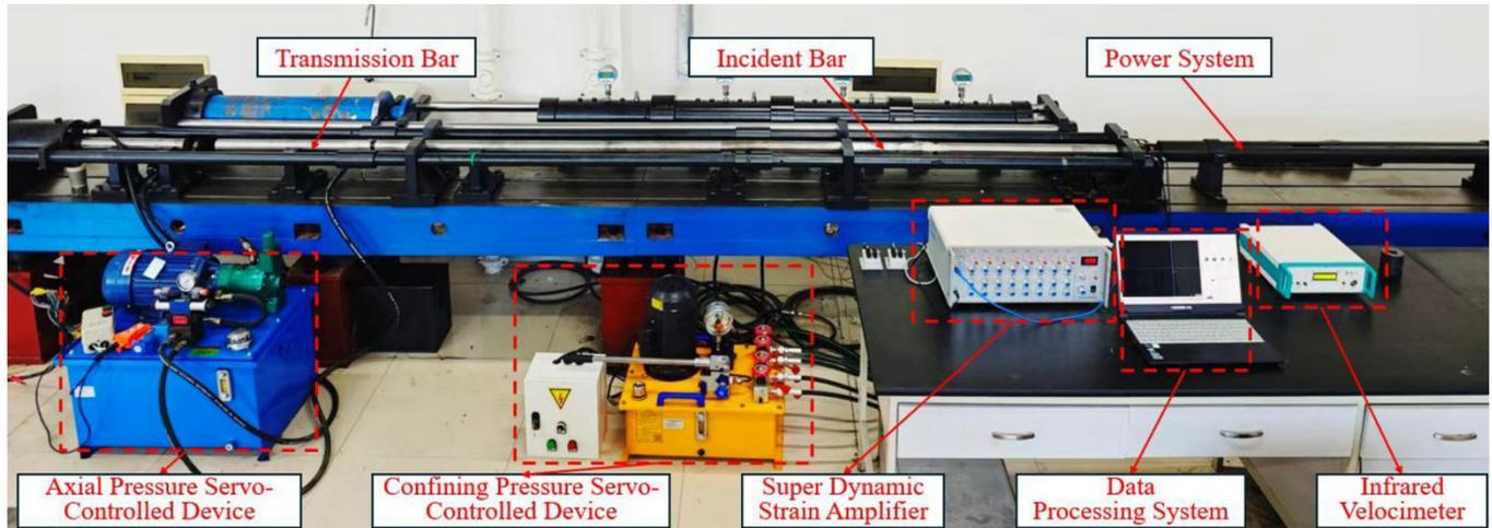
Figure 2. Split Hopkinson Pressure Bar (SHPB) impact testing system
