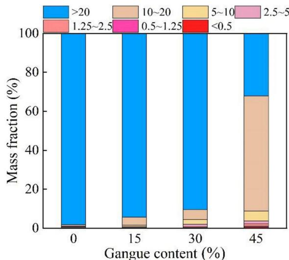
**Figure 11.** Mass distribution of specimens subjected to 0.1 MPa cyclic impact
