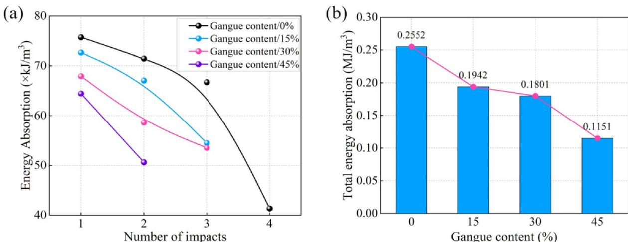
**Figure 10.** Energy absorbed of CGC under cyclic impact: **a** energy absorbed per impact, **b** total energy absorbed
