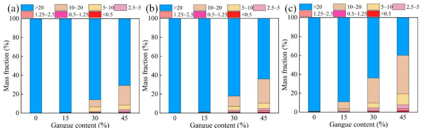
**Figure 7.** Particle size distribution of specimen fragmentation under single impact: **a** impact gas pressure 0.35 MPa, **b** impact pressure 0.45 MPa, **c** impact pressure 0.55 MPa
