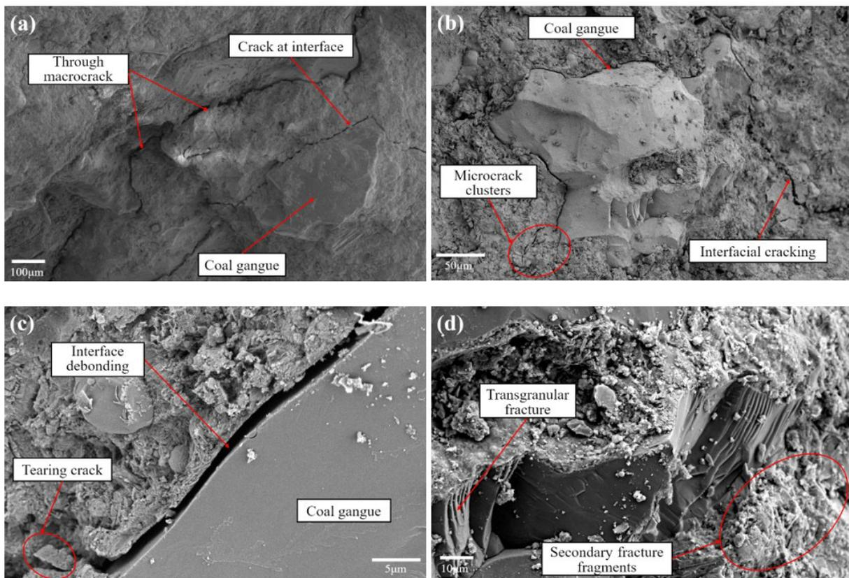
**Figure 12.** Microstructure of typical specimens: **a** lateral crack propagation along CG ( $\times 100$ ), **b** peripheral crack development around CG ( $\times 300$ ), **c** debonding at the cg–matrix interface ( $\times 3000$ ), **d** fracture morphology of CG ( $\times 1000$ )
