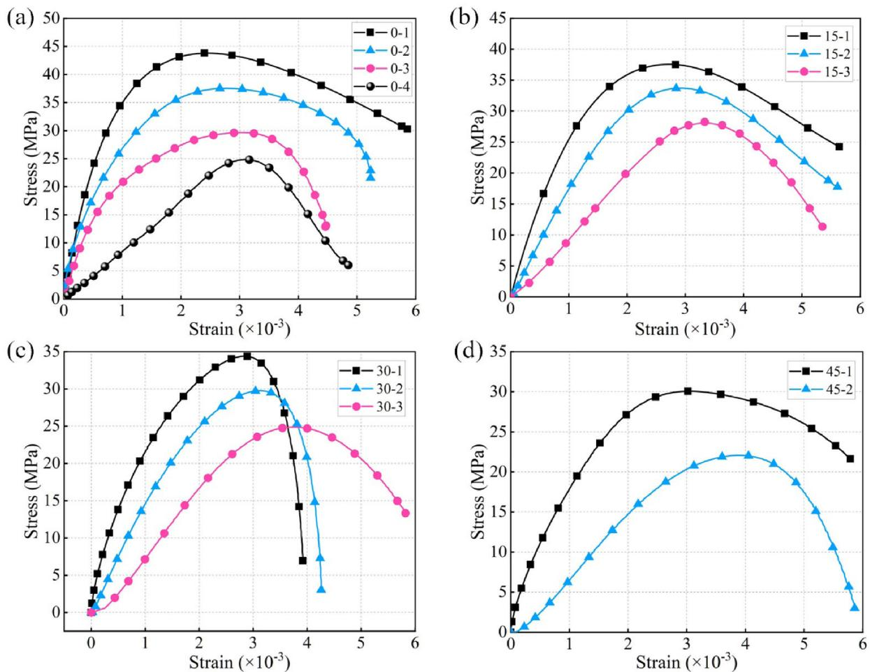
**Figure 8.** Stress-Strain Curves of CGC under Cyclic Impact: **a** CG Content 0%, **b** CG Content 15%, **c** CG Content 30%, **d** CG Content 45%
