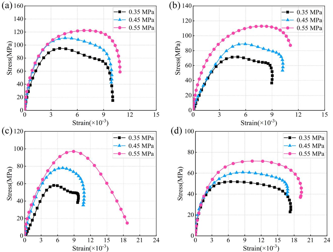
Figure 4. Stress-strain curves of specimens under single impact: a content 0%, b content 15%, c content 30%, d content 45%
