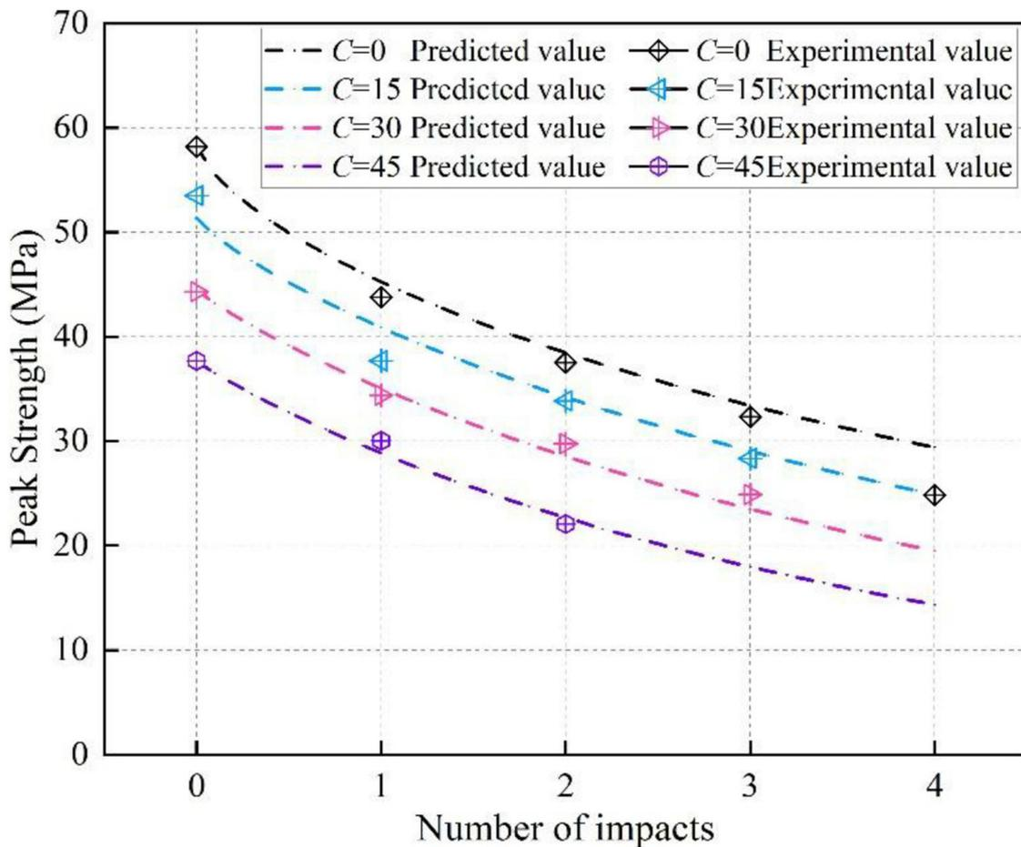
**Figure 13.** Comparison of results from the impact performance degradation model for CGC
