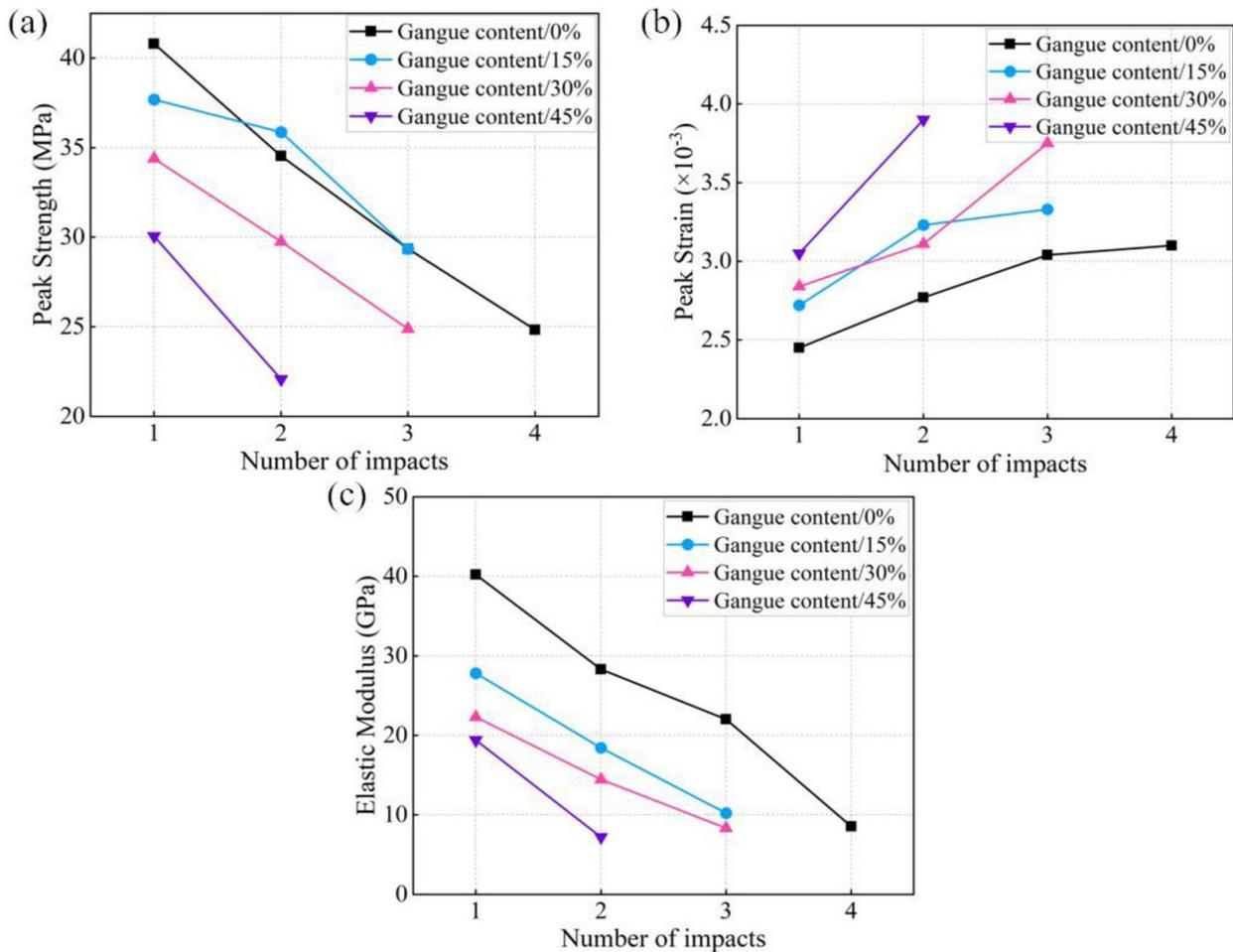
**Figure 9.** Evolution of mechanical properties of CGC under cyclic impact: **a** peak strength, **b** peak strain, **c** elastic modulus
