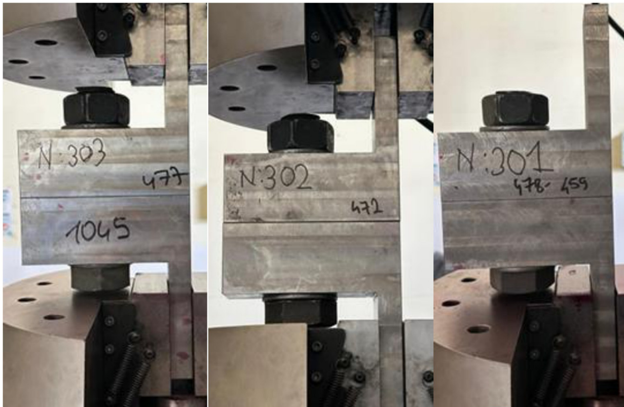
Figure 7 Pre-fatigue test appearance of N301, N302, N303 specimens.
