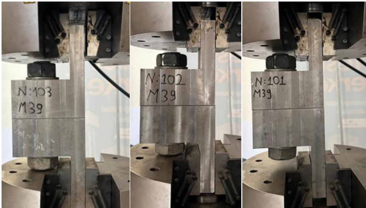
Figure 5 Pre-fatigue test appearance of N101, N102, N103 specimens with M39 bolts.
