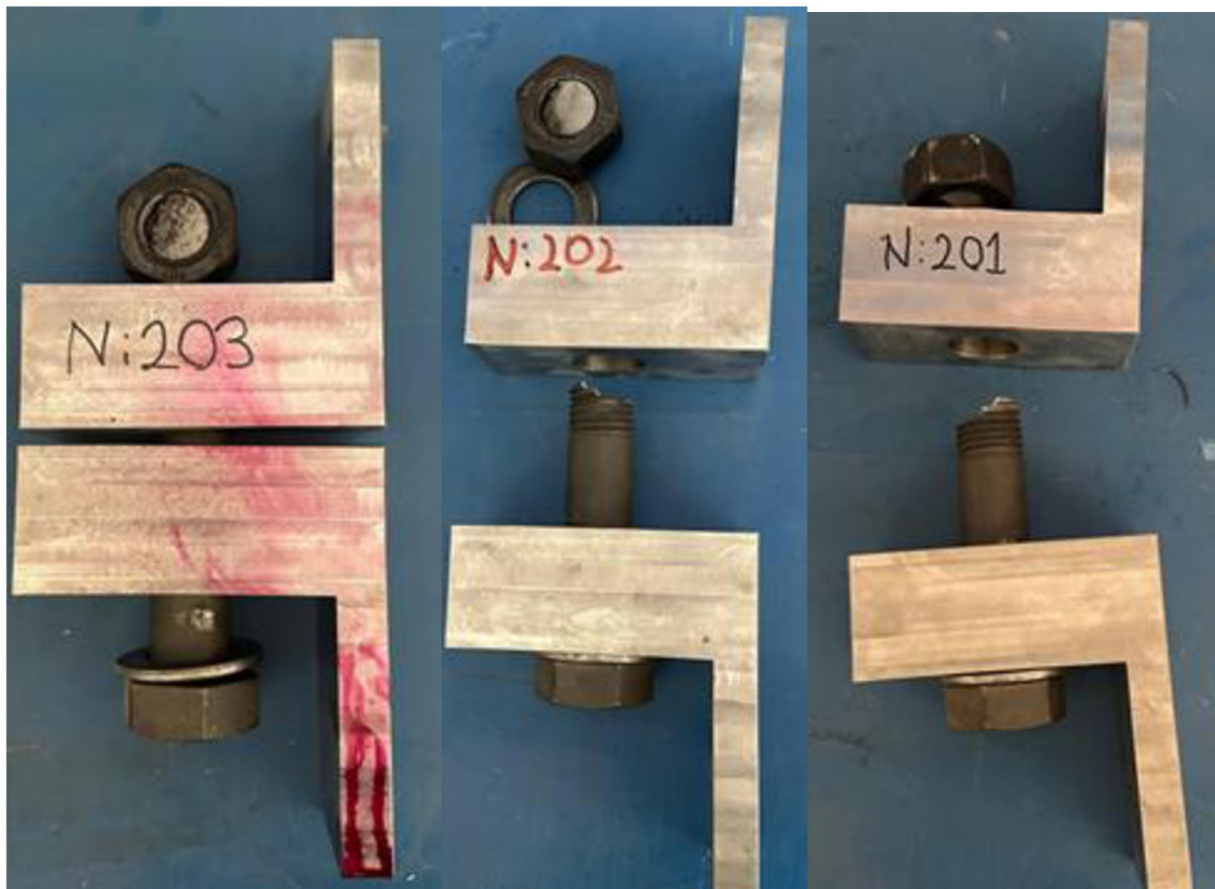
Figure 11 Post-fatigue test appearance of N201, N202, N203 specimens.
