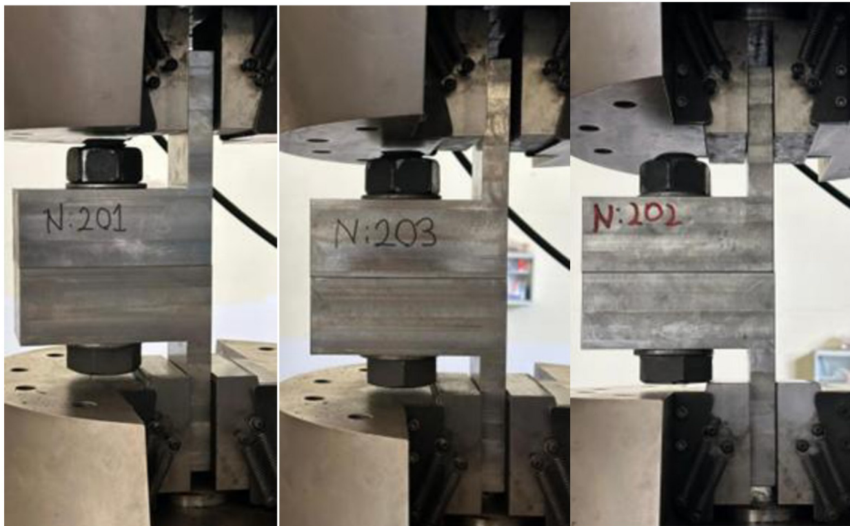
Figure 10 Pre-fatigue test appearance of N201, N202, N203 specimens.
