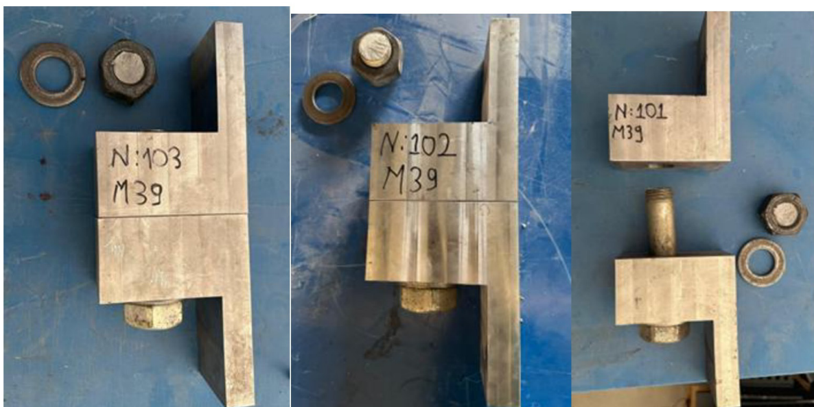
Figure 6 Post-fatigue test appearance of N101, N102, N103 specimens with M39 bolts.
