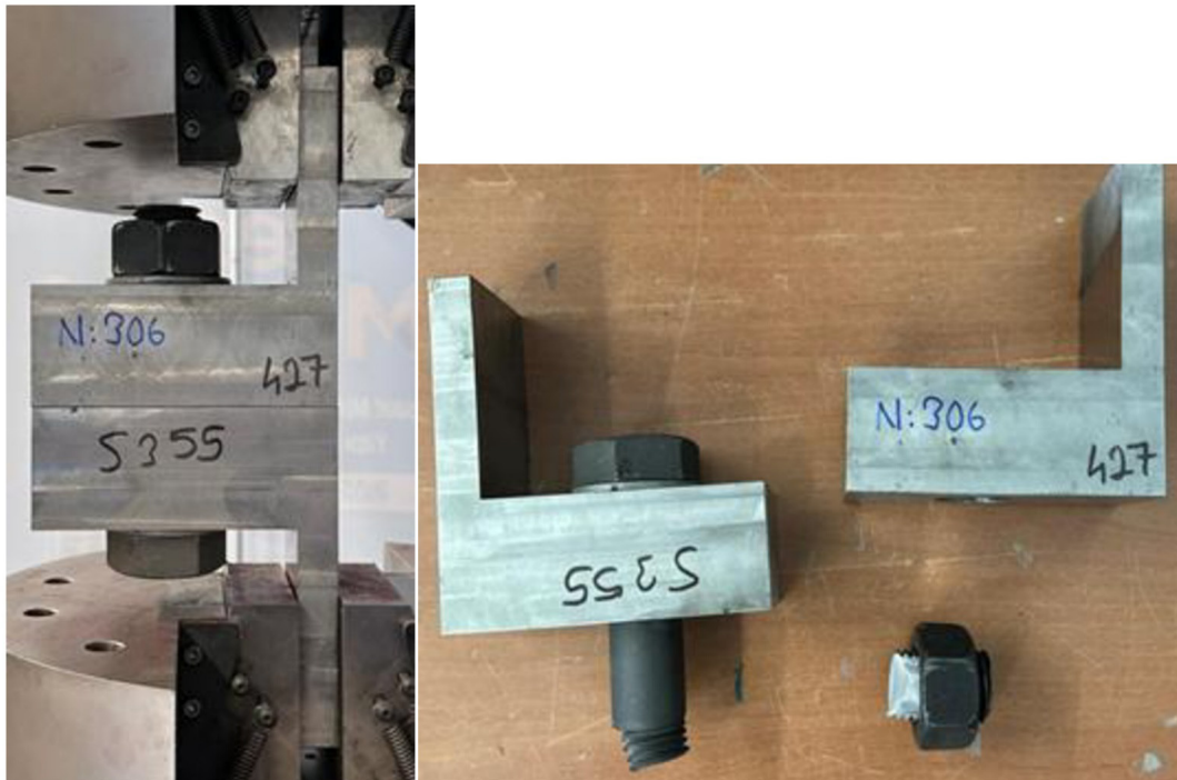
Figure 9 Pre and Post fatigue test appearance of N306 specimens.
