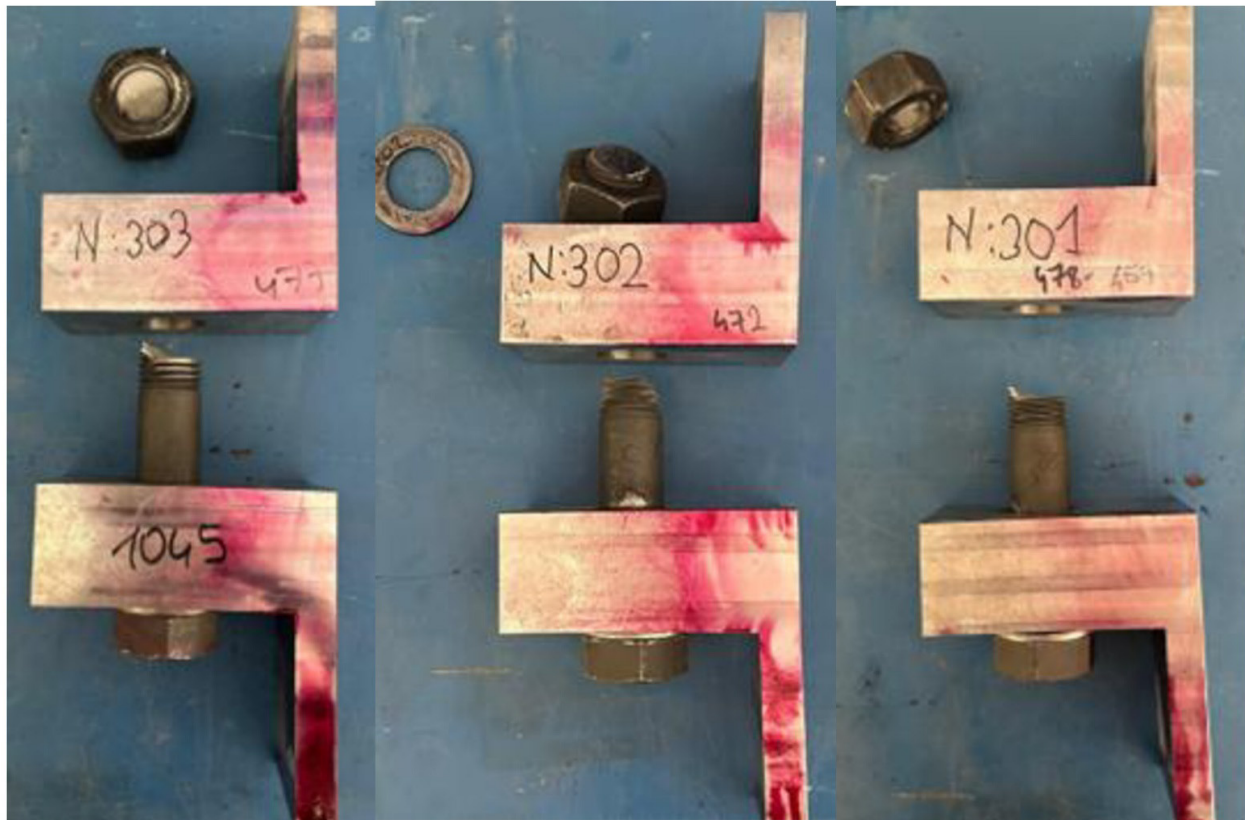
Figure 8 Post-fatigue test appearance of N301, N302, N303 specimens.
