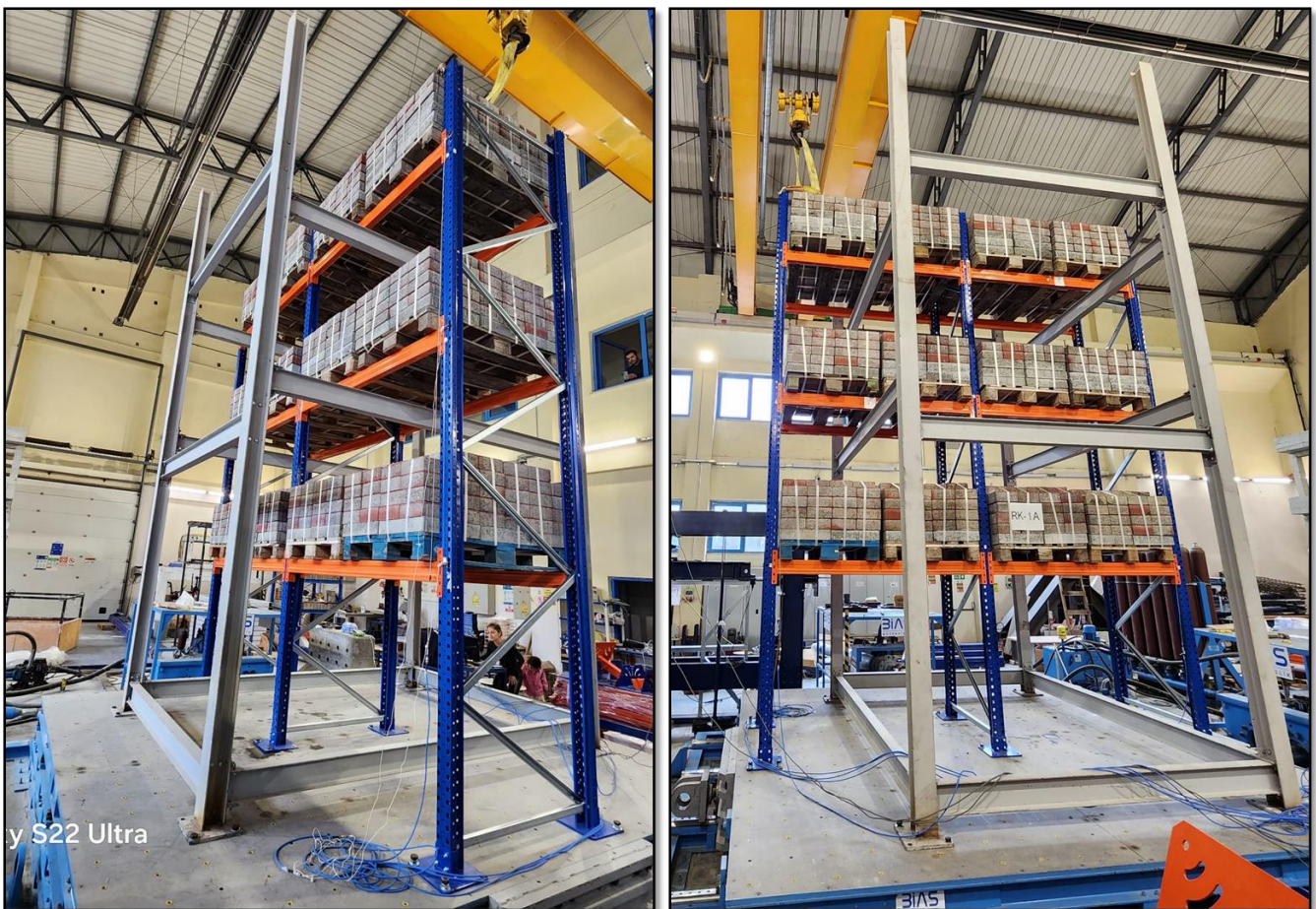
Figure 5 Shaking table test setup of cold-formed rack system.
