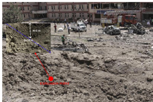
Figure 10 Forensic field measurements of the crater geometry formed at the explosion site
