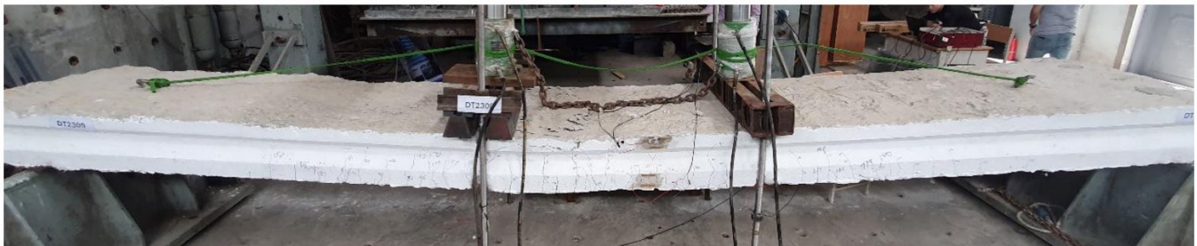
Figure 9 Failure mode and crack pattern structure of BC1 beam
