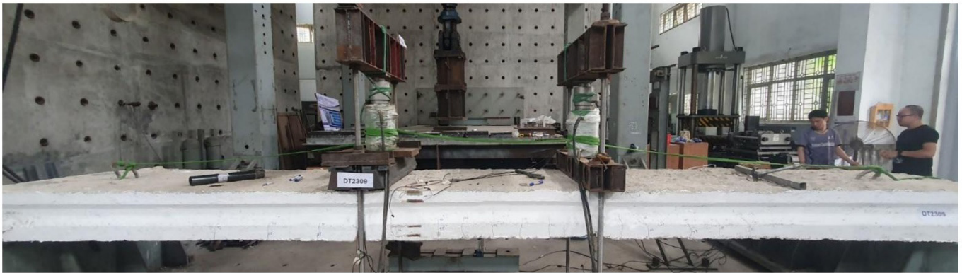
Figure 10 Crack pattern of BC2 during preloading and sustained loading
